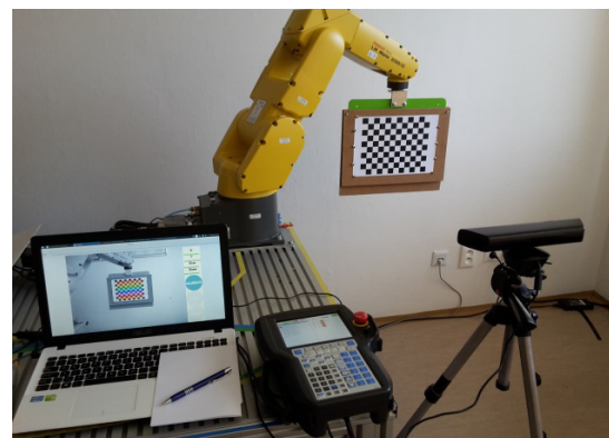
Fig. 3. Calibration of RGB and IR cameras intrinsic parameters; a) the calibration pattern with a checkboard pattern; b) the calibration workplace with robot Fanuc
