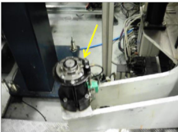
Fig. 6. Inserted bearing on the press head
