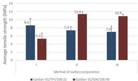
Fig. 4. The bonded joints shear tensile strength of 1.4310 sheets
