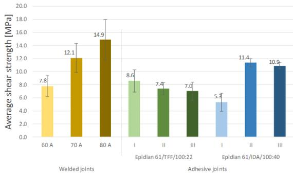
**Fig. 5.** Comparison of shear strength of welded and bonded joints of 1.4310 acid-resistant steel sheets
