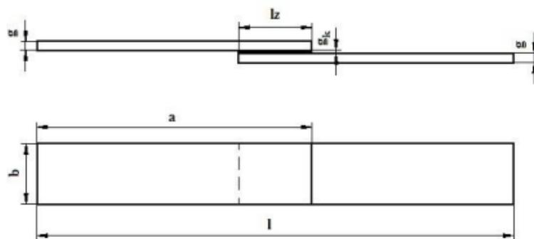
Fig. 2. The bonded joint of 1.4310 sheet
