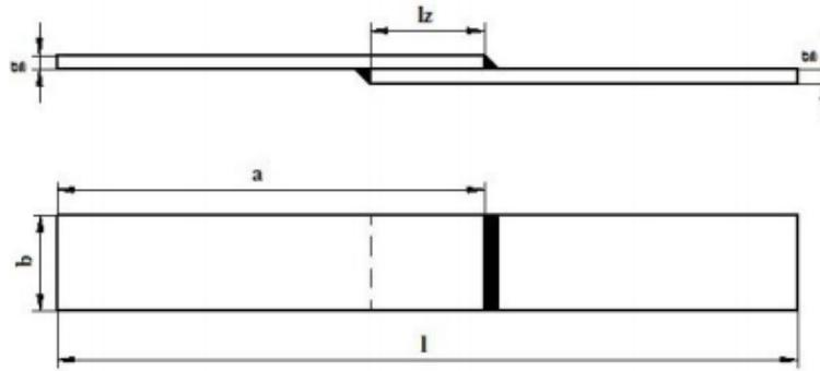
Fig. 1. The welded joint of 1.4310 sheet
