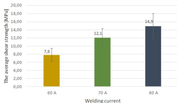
Fig. 3. The welded joints on shear strength of 1.4310 acid-resistant steel sheets
