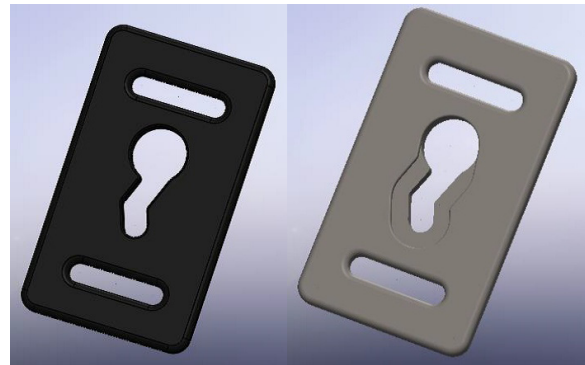
Fig. 1. Original (left) and modified (right) design of a clip for slings in medical lifts
