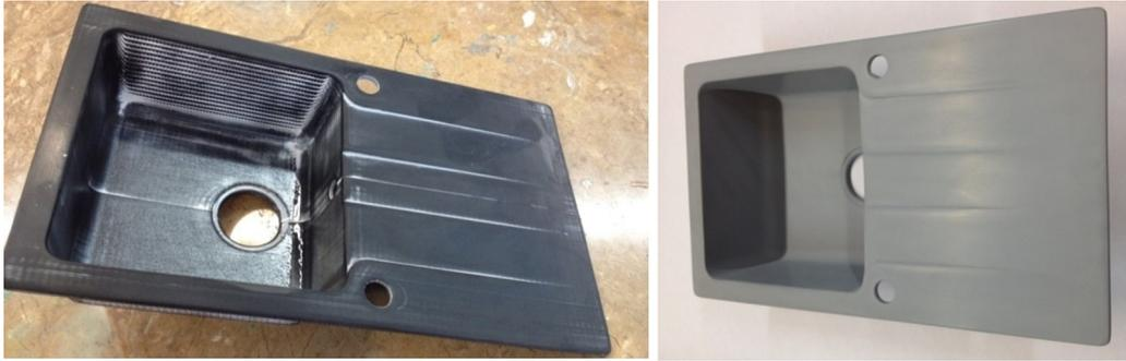
**Fig. 7.** Product after puttying and sanding (left) and after putting priming paint
