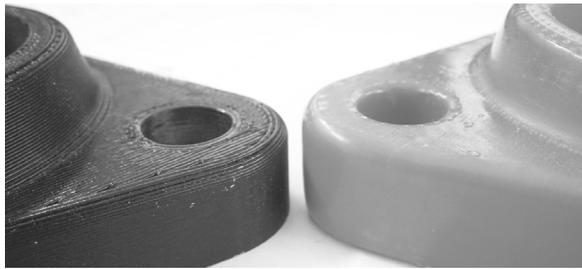
**Fig. 3.** Effect of smoothing a surface of ABS part with acetone vapors
