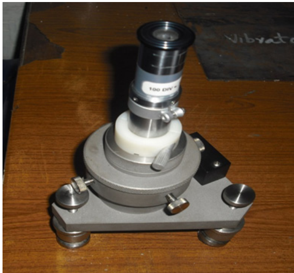
Fig. 2. Hole-drilling apparatus used for determination of residual stresses below the surface at different depths: left – milling guide, right – data logger
