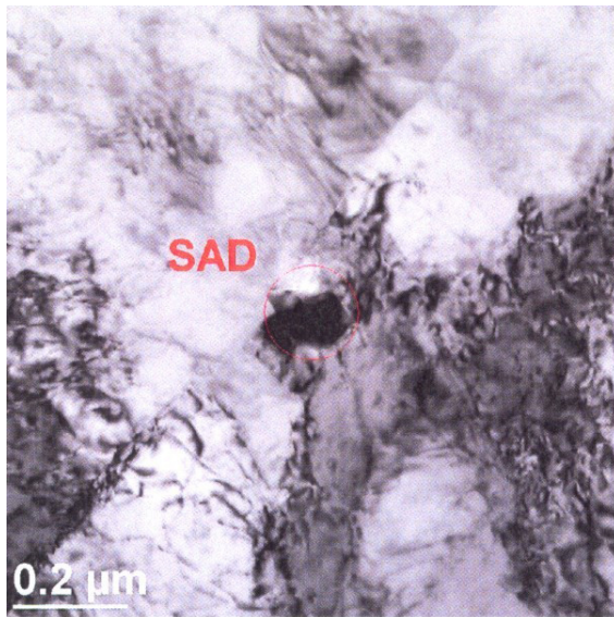
Fig. 3. Microstructure of the zinc and iron interlayer (a) and the stoichiometric analysis of the Fe_2Al phase (b) obtained on a zinc coating obtained from a zinc bath modified with aluminium and magnesium
