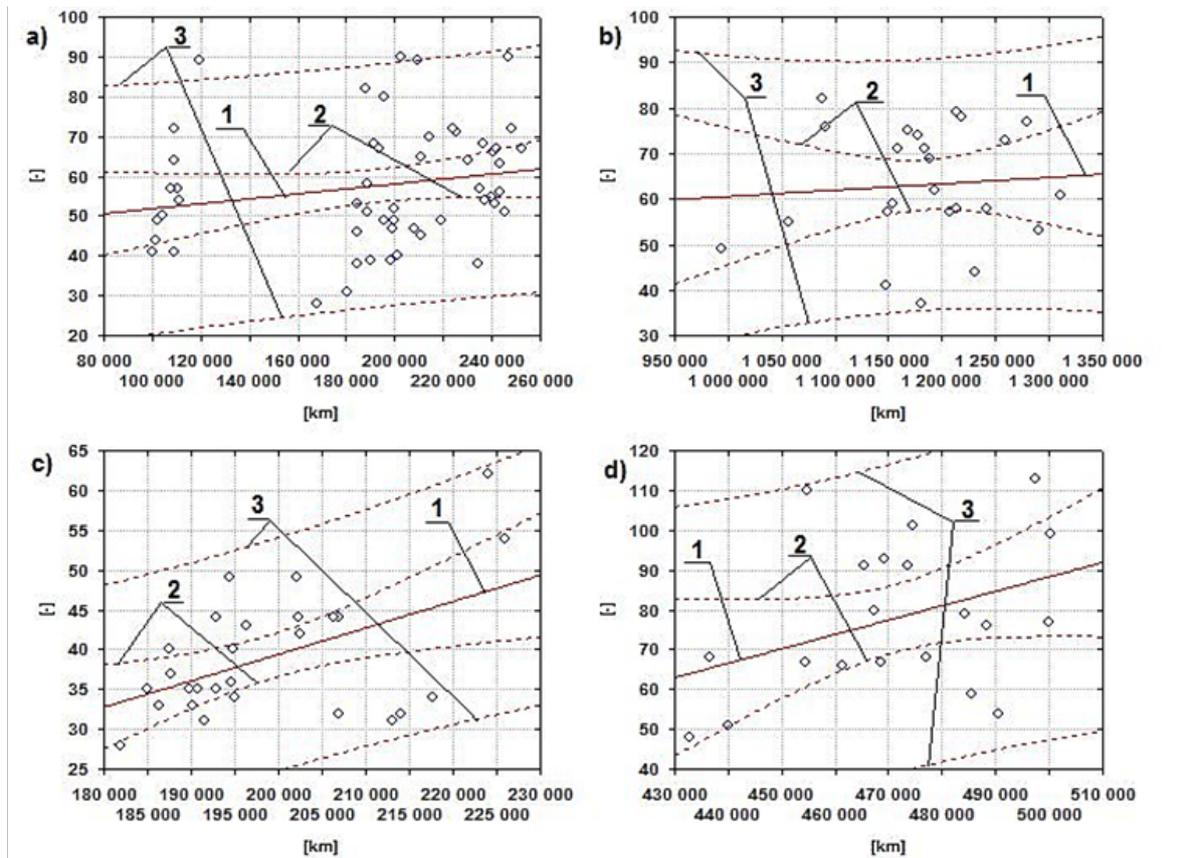
**Fig. 1.** The chart of dispersion and the regression line between the initial kilometrage and the annual number of orders at the maintenance and service system of the examined units for buses; a) Autosan, b) Jelcz, c) Mercedes, d) Solaris, 1 - regression line, 2 - confidence interval for the forecasted average observation, 3 - confidence interval for the forecasted observation
