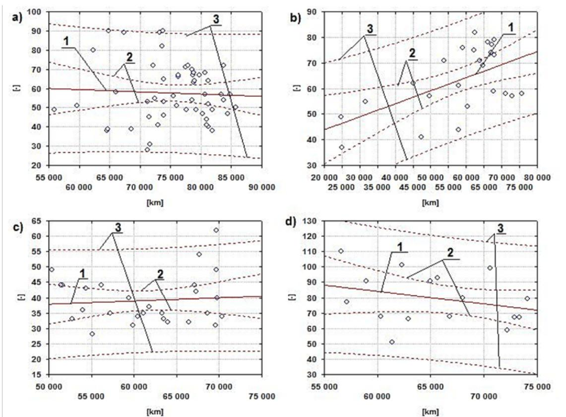
**Fig. 2.** The chart of dispersion and the regression line between the annual kilometrage and the annual number of orders at the maintenance and service system of the examined units for buses; a) Autosan, b) Jelcz, c) Mercedes, d) Solaris, 1 - regression line, 2 - confidence interval for the forecasted average observation, 3 - confidence interval for the forecasted observation
