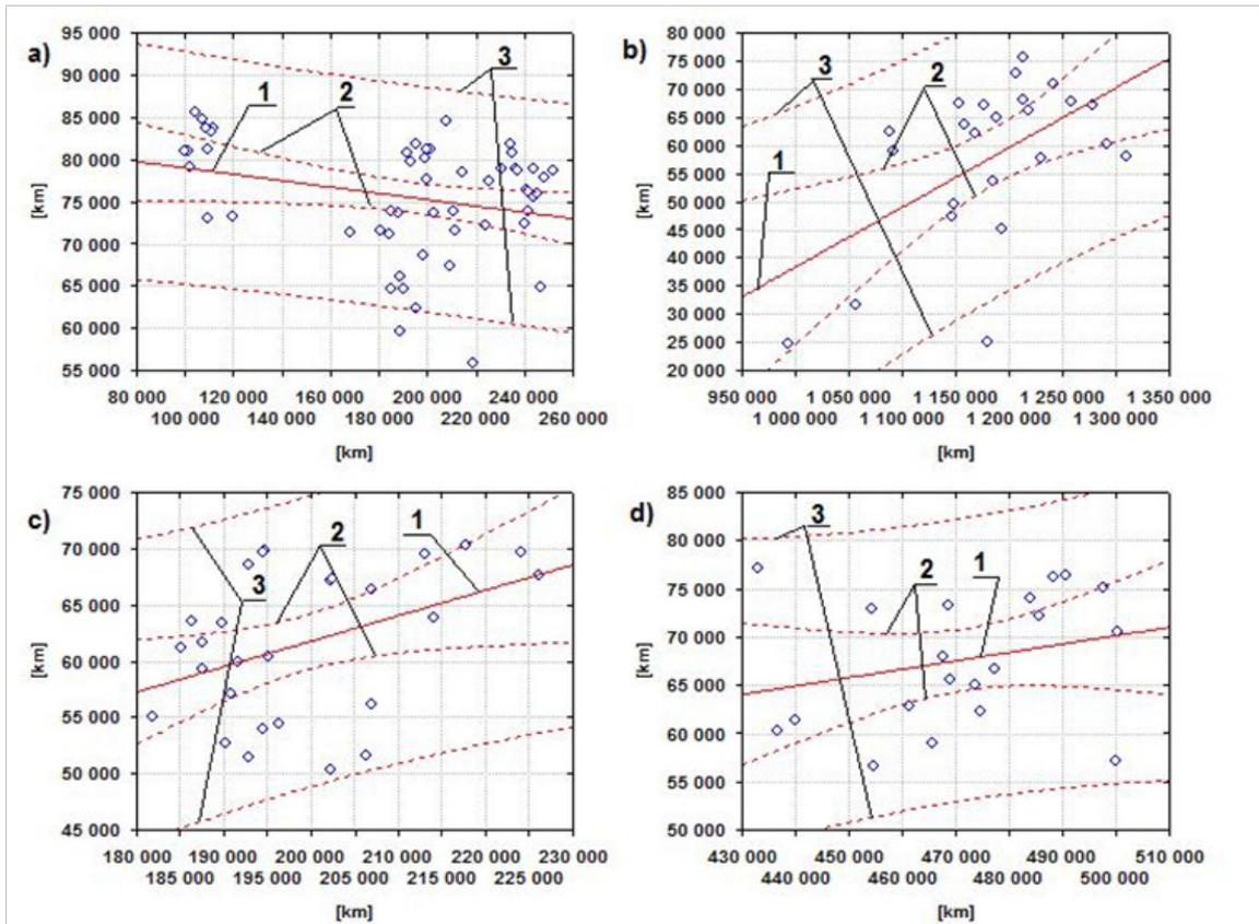
**Fig. 3.** The chart of dispersion and the regression line between the annual and the initial kilometrage for buses: a) Autosan, b) Jelcz, c) Mercedes, d) Solaris, 1 - regression line, 2 - confidence interval for the forecasted average observation, 3 - confidence interval for the forecasted observation
