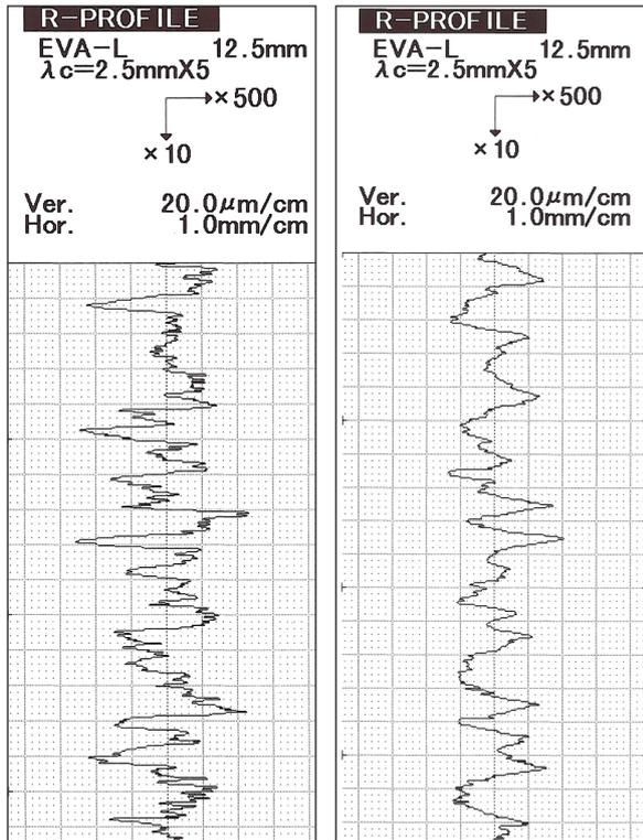
Fig. 5. Roughness graphs of surface machined with rotary tool:  $\lambda_s = 30^\circ$ ,  $f = 0.45$  mm (left) and  $\lambda_s = 50^\circ$ ,  $f = 0.9$  mm (right)
