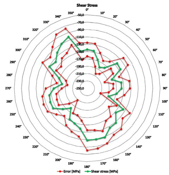
Fig. 11 Shear stress graph with cutting parameters  $\lambda_s = 50^\circ$ ,  $f=0,9$ mm
