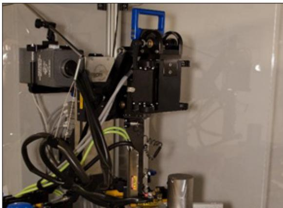
Fig. 3. Process of residual stress measurement with XRD diffractometer
