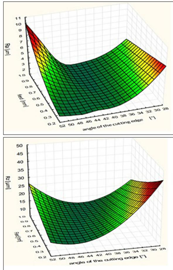
Fig. 6. Roughness parameter Ra in turning with auto-rotary tool (above) and roughness parameter Rz in turning with auto-rotary tool (below)
