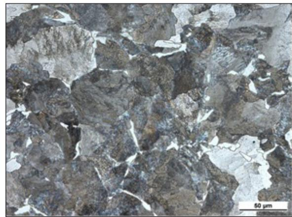
**Fig. 4.** Microstructure of bearing steel 100Cr6
