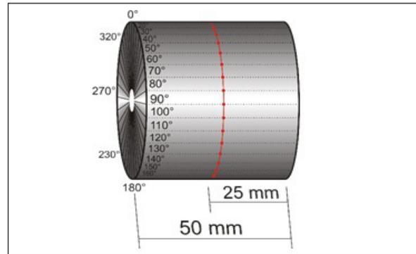
Fig. 7. Position of measured points for X-ray diffraction
