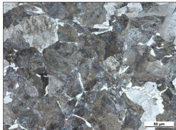
Fig. 4. Microstructure of bearing steel 100Cr6
