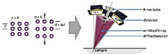
Fig. 1. Principle of measuring of residual stress by X-ray diffractometry based on Bragg's Law [5]
