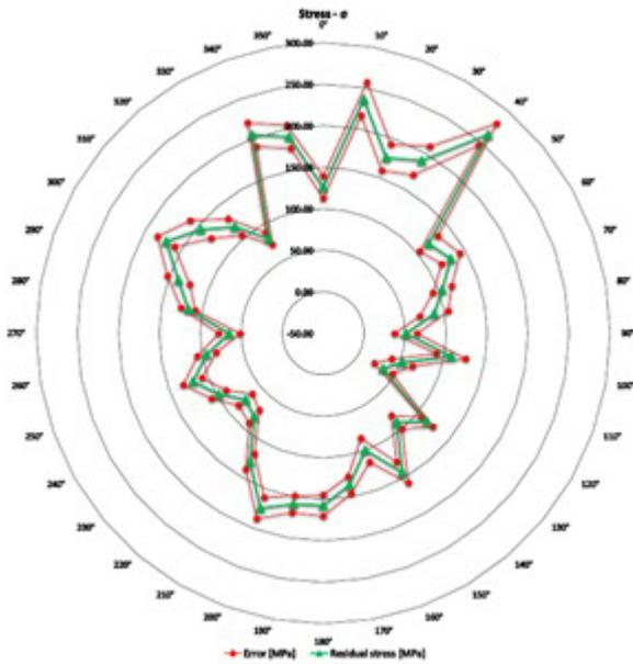
Fig. 8. Residual stress graph with cutting parameters  $\lambda_s = 30^\circ$ ,  $f=0,45$  mm
