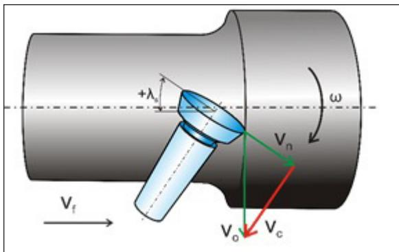
Fig. 2. Tool position relative to workpiece, negative angle  $\lambda_s$  [13]
