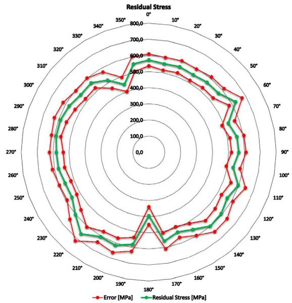
Fig. 10. Residual stress graph with cutting parameters  $\lambda_s = 50^\circ$ ,  $f=0,9$  mm
