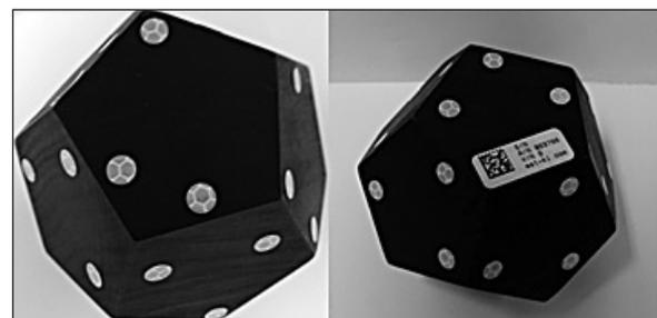
**Fig. 4.** A reference object – regular dodecahedron with the optical system markers, supplied by the PST-55 device manufacturer
