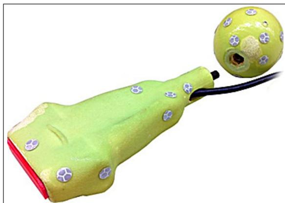
**Fig. 3.** Physical model of a modified ultrasound examination head, with the additional object – a surface for additional markers. Retroactive markers of the PST-55 system arranged on the basic and additional geometry
