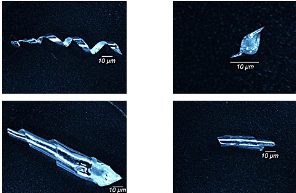
**Fig. 4.** Chips formed in AZ91HP magnesium cast alloy milling for selected chip fractions and depths of cut  $a_p$  ( $f_z = 0.05$  mm/tooth): a)  $a_p = 0.5$  mm, fraction A, b)  $a_p = 0.5$  mm, fraction C, c)  $a_p = 3$  mm, fraction A, d)  $a_p = 3$  mm, fraction B
