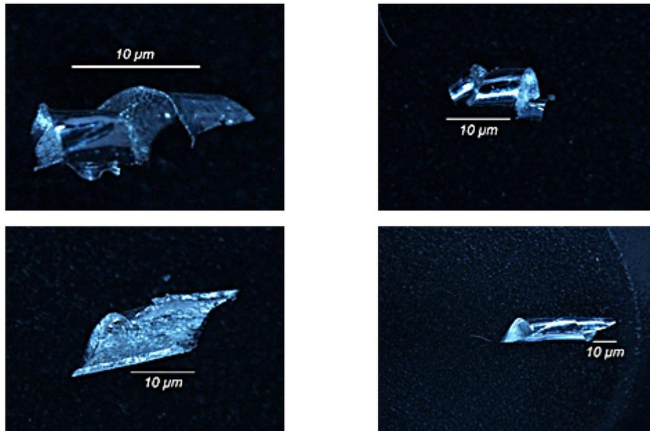
**Fig. 5.** Chips formed in AZ91HP magnesium cast alloy milling for selected chip fractions and depths of cut  $a_p$  ( $f_z = 0.15$  mm/tooth): a)  $a_p = 0.5$  mm, fraction C, b)  $a_p = 1.5$  mm, fraction D, c)  $a_p = 1.5$  mm, fraction C, d)  $a_p = 3$  mm, fraction C
