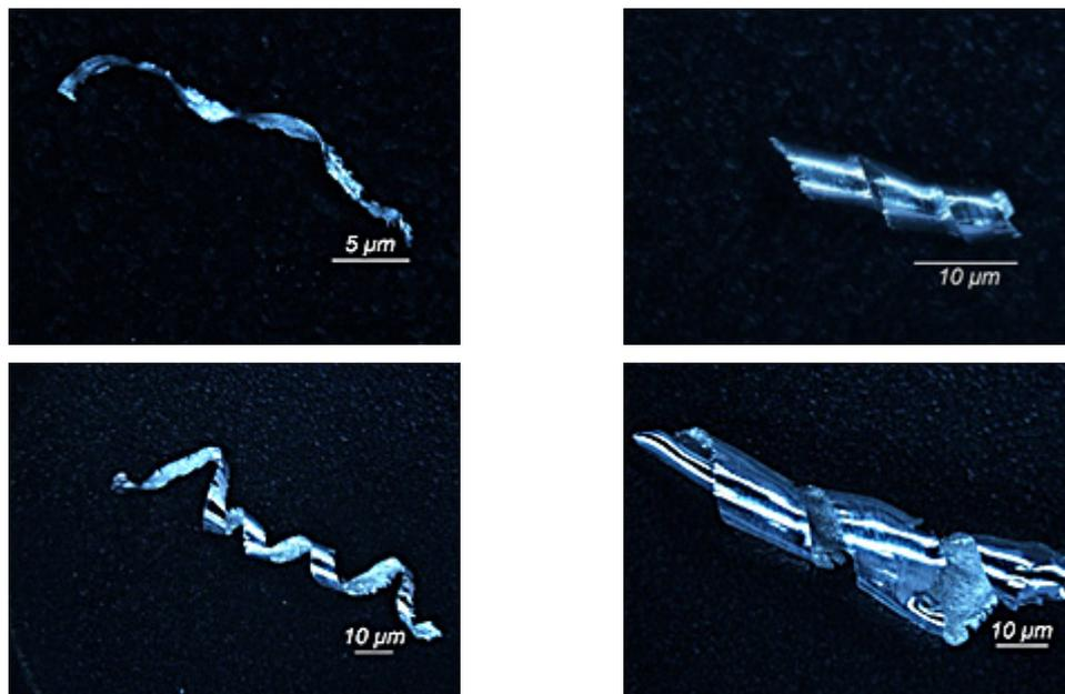
**Fig. 2.** Chips formed in AZ91HP magnesium cast alloy milling for selected chip fractions and depths of cut  $a_p$  ( $f_z = 0.05$  mm/tooth): a)  $a_p = 0.5$  mm, fraction D, b)  $a_p = 0.5$  mm, fraction C, c)  $a_p = 0.5$  mm, fraction A, d)  $a_p = 1.5$  mm, fraction A
