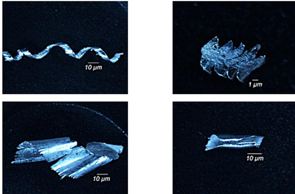
**Fig. 3.** Chips formed in AZ91HP magnesium cast alloy milling for selected chip fractions and depths of cut  $a_p$  ( $f_z = 0.15$  mm/tooth): a)  $a_p = 0.5$  mm, fraction A, b)  $a_p = 0.5$  mm, fraction C, c)  $a_p = 3$  mm, fraction A, d)  $a_p = 3$  mm, fraction D
