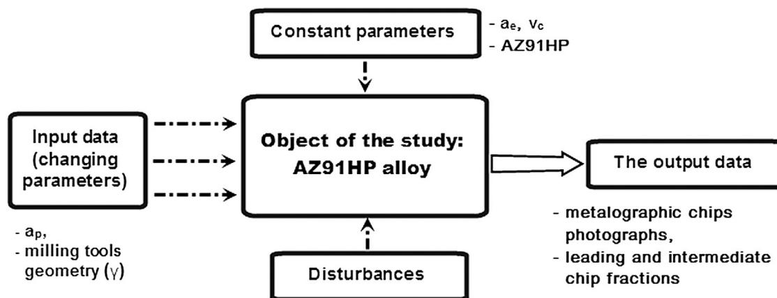
Fig. 1. Test plan for assessment of  $a_p$  and  $\gamma$  impact on chip form
