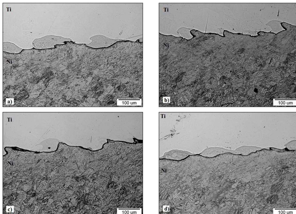
Fig. 2. Microstructure of the explosion welded Ni / Ti joints, 200 $\times$
