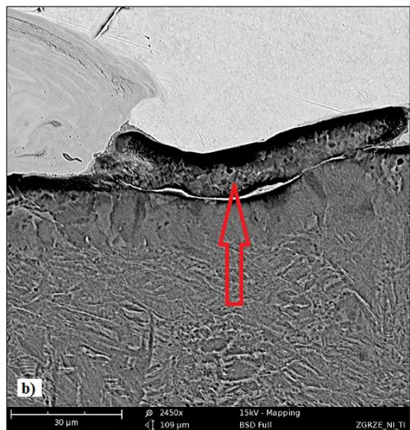
**Fig. 5.** SEM micrographs of the explosion welded Ni / Ti joints,
