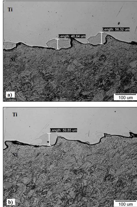
**Fig. 4.** Wave height in the cross section of the explosion welded Ni / Ti joints, 200×,
