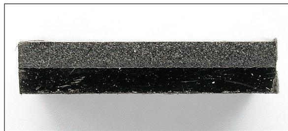
Fig. 1. Cross-section of the explosion welded joint (top layer – Ti, bottom layer – Ni)
