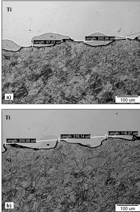
**Fig. 3.** Wave length in the cross section of the explosion welded Ni / Ti joints, 200×,
