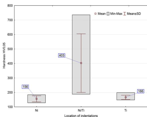
Fig. 6. Microhardness results of the Ni/Ti interface and base materials
