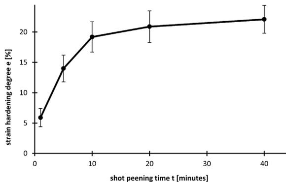
Fig. 6. Effect of shot peening time onto strain hardening degree
