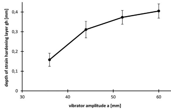
Fig. 7. Effect of vibrator amplitude onto depth of strain hardening layer
