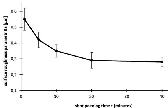
Fig. 3. Effect of shot peening time onto Ra surface roughness parameter
