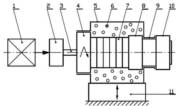
**Fig. 1.** Schematic illustration of the stand for vibratory and rotational shot peening: 1 – electric motor, 2 – reduction gear, 3 – flexible coupling, 4 – spindle, 5 – working chamber, 6 – bead, 7 – sample, 8, 10 – special nuts, 9 – slide bearing, 11 – vibrator
