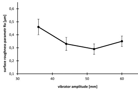
Fig. 2. Effect of vibrator amplitude onto Ra surface roughness parameter
