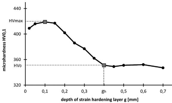
Fig. 4. Typical surface layer microhardness distribution after vibratory and rotational shot peening
