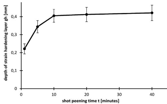
Fig. 8. Effect of shot peening time onto depth of strain hardening layer
