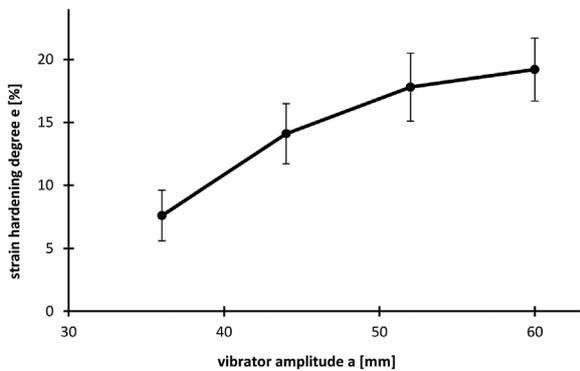
Fig. 5. Effect of vibrator amplitude onto strain hardening degree
