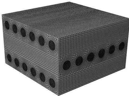
Fig. 1. FEM mesh for multi-layered composite
