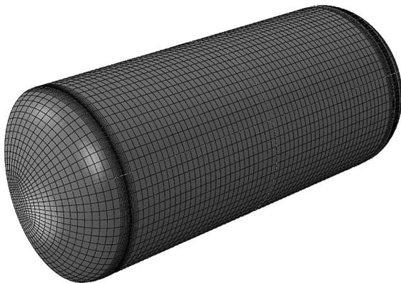
Fig. 4. Model of cylindrical vessel under internal pressure
