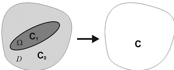
Fig. 2. Heterogeneous material (left) and equivalent homogeneous material (right)
