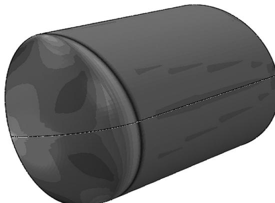
Fig. 6. Maximum effective stress [Pa] in pressure vessel
