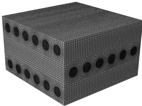
Fig. 1. FEM mesh for multi-layered composite
