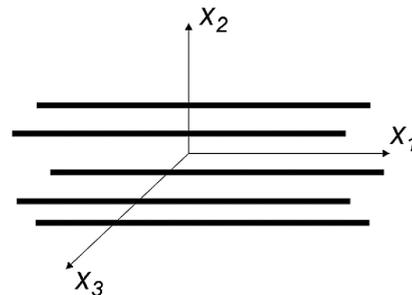
Fig. 3. Model of unidirectional fiber-reinforced composite
