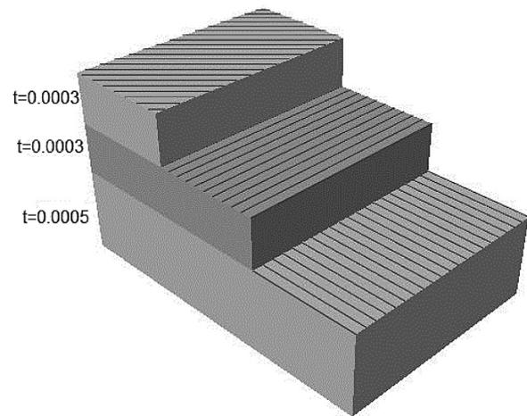
Fig. 5. Composite layers and thicknesses [mm]
