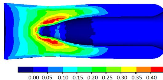
Fig. 4. Distribution of damage function according to Cockroft-Latham criterion for time  $t = 7$  s
