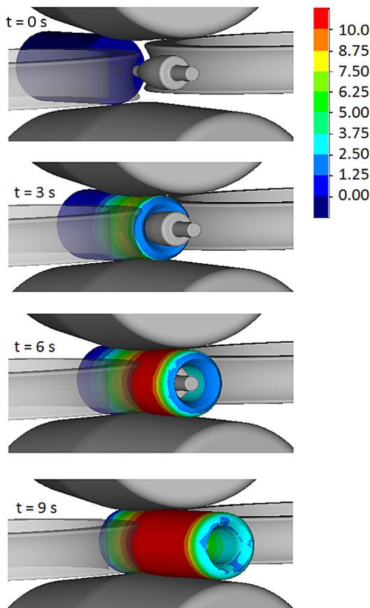
Fig. 3. Progression of the workpiece shape in the piercing process with marked distribution of effective strain
