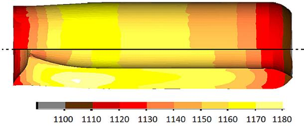
Fig. 5. Distribution of temperature in the bush at the end of piercing process (for  $t=10$  s)
