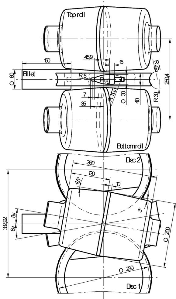
Fig. 1. Schematic view a of the analyzed numerically piercing process of a thick-walled bush
