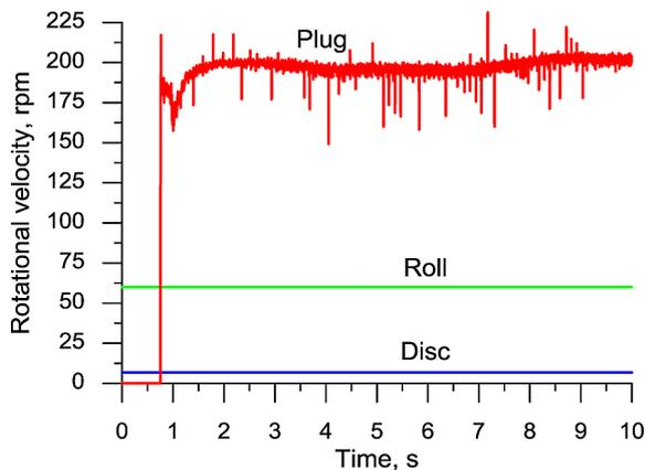
Fig. 6. Rotational velocities of tools in the analyzed piercing process
