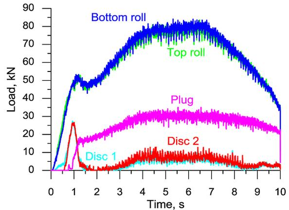
Fig. 7. Forces acting on tools in the piercing process, marked according to Figure 1
