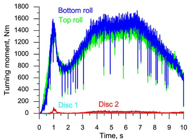
Fig. 8. Turning moments acting on tools in the piercing process, marked according to Figure 1
