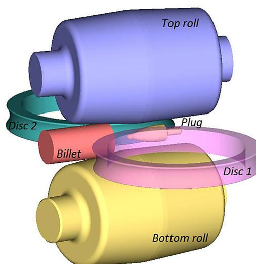
Fig. 2. FEM model of the piercing process of a thick-walled bush
