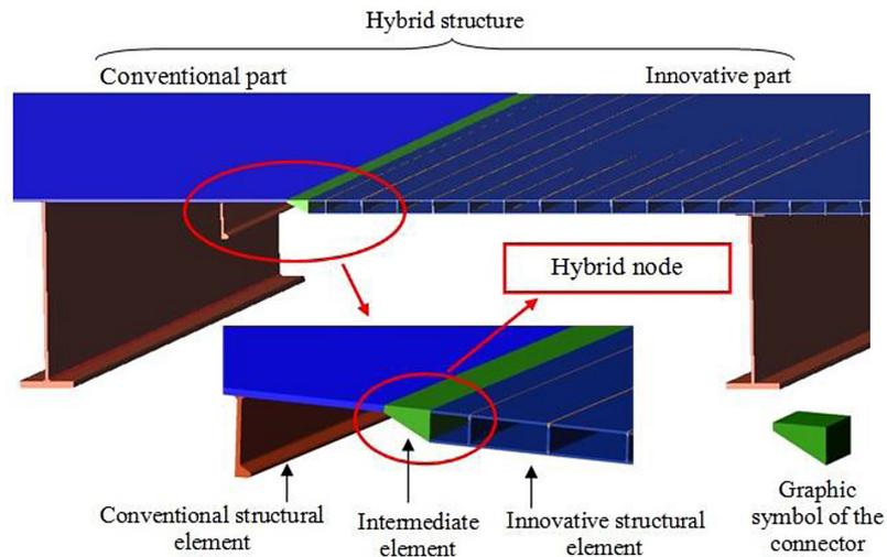
Fig. 1. Hybrid node – components [5, 6]
