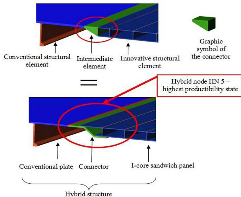
**Fig. 4.** The hybrid node characterized by the highest state of productibility (on the basis of [5])
