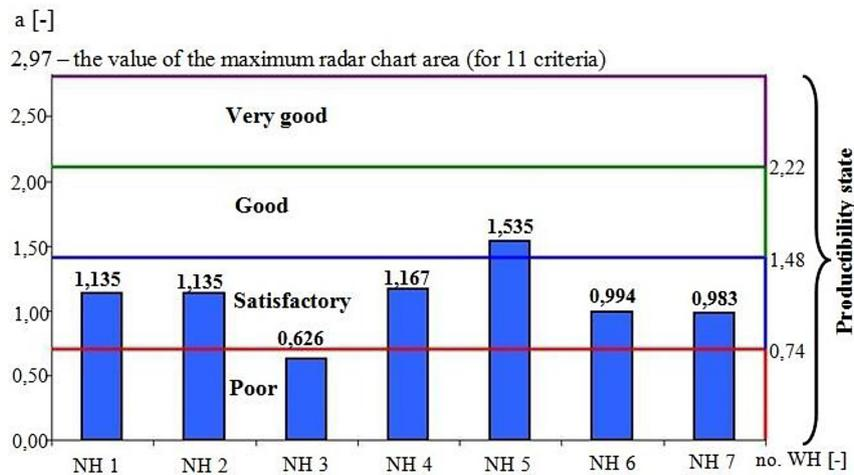
Fig. 3. A comparison of the radar chart area values describing the productivity of the hybrid nodes assessed (on the basis of [5])
