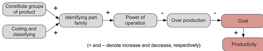
**Fig. 1.** The impact of part family (grouping, classifying and coding) on manufacturing system – Extracted and modified from Ham et al. [1985]
