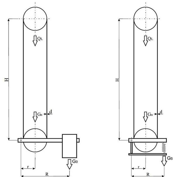
Fig. 6. Geometry of braking system in a frictional lift: R – length of the arm of the effect of force exerted by tension  $G_o$  (spring  $G_s$ ) [m],  $r$  – length of the arm of the effect of straining force  $G_n$  [m],  $G_o$  – weight of the tension [kg],  $d$  – diameter of limiter rope [m],  $Q_i$  – weight of the rope resulting from lifting height [kg]
