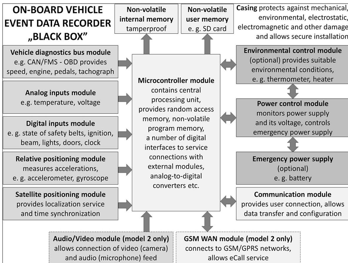
Fig. 4. On-board vehicle, event data recorder functional structure [G. Nowacki, A. Niedzicka]
