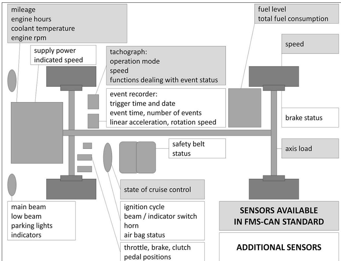
Fig. 3. Monitoring sensors in vehicle [8]
