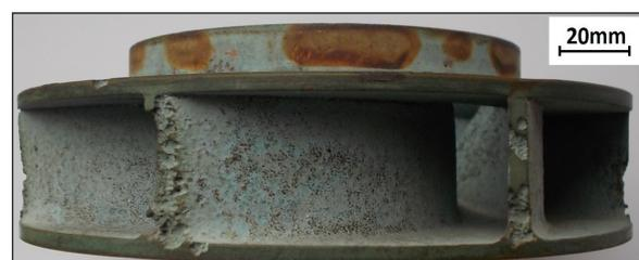
Fig. 1. Radial impeller worn by cavitation
