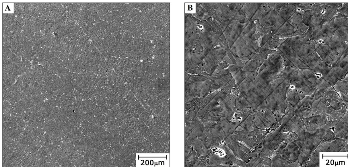
Fig. 10. SEM micrographs of coating 9, after 120 minutes of cavitation test
