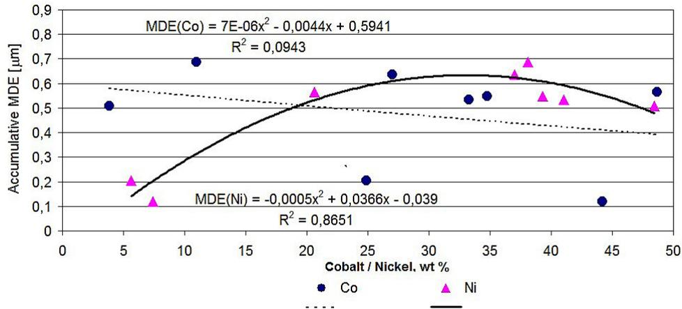
Fig. 5. Accumulative MDE parameters of coatings 2–5, 7–10, after 120 minutes of cavitation, with relation to their main matrix elements
