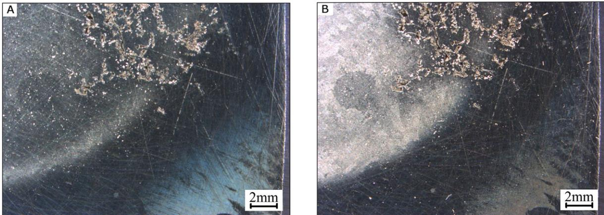
Fig. 6. Coating 6: A – after 30 minutes and B – after 120 minutes of cavitation test
