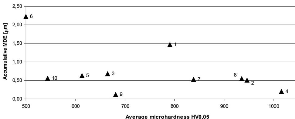
Fig. 9. Accumulative MDE after 120 minutes of cavitation versus the range of microhardness of coatings (1-10)
