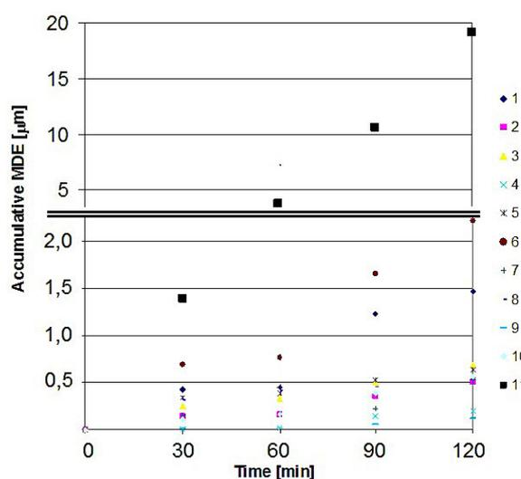
Fig. 4. Cavitation erosion resistance of coatings (1–10) and reference sample (11)
