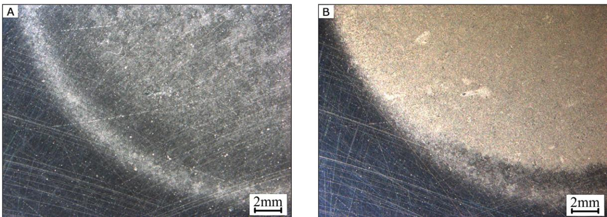
Fig. 7. Coating 5: A – after 30 minutes and B – after 120 minutes of cavitation test
