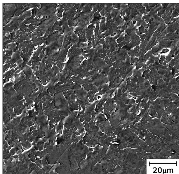
Fig. 11. SEM micrograph of coating 6 after 120 minutes of cavitation test
