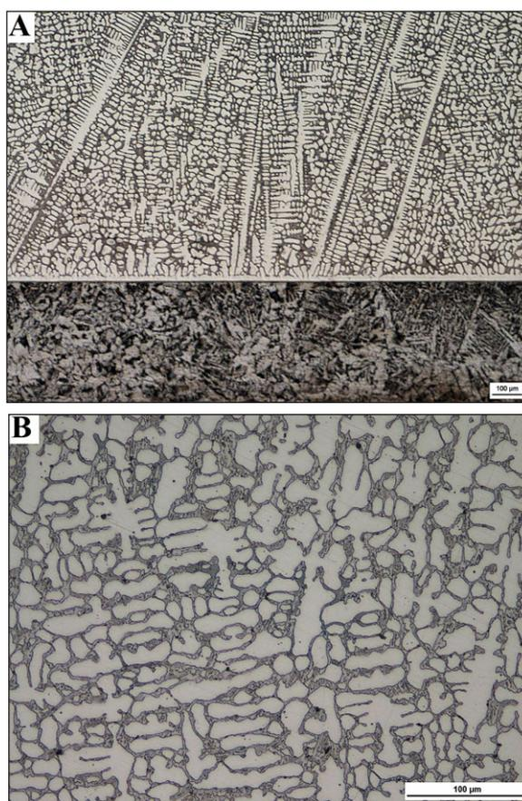
Fig. 3. LOM micrographs. The cross-section of sample 3 (A) and microstructure of coating 9 (B)
