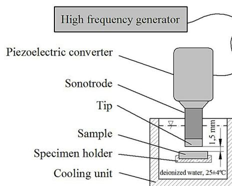
**Fig. 2.** Schematic diagram of the ultrasonic equipment
