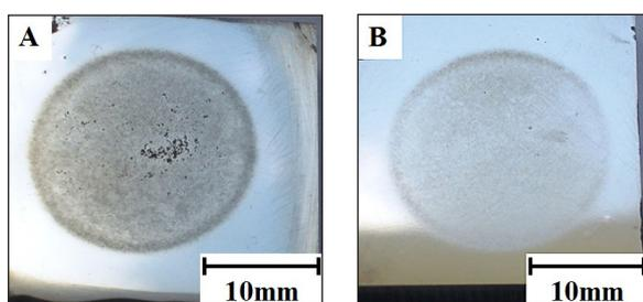
Fig. 8. Specimen surface after 120 minutes of cavitation: A – coating 3; B – coating 2
