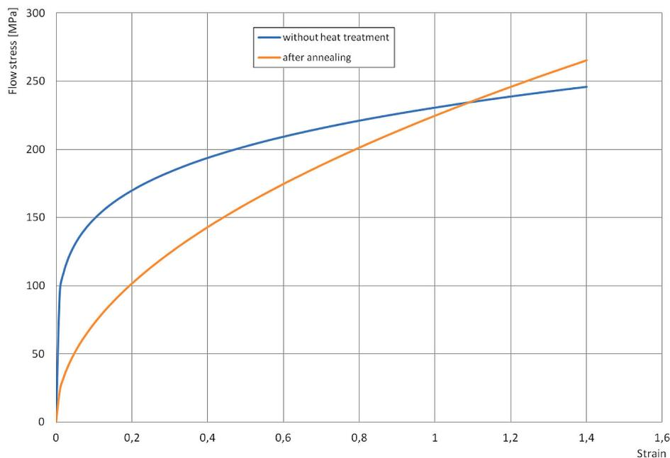
**Fig. 5.** Comparison of the flow curves described by the determined equations (3) and (4)
