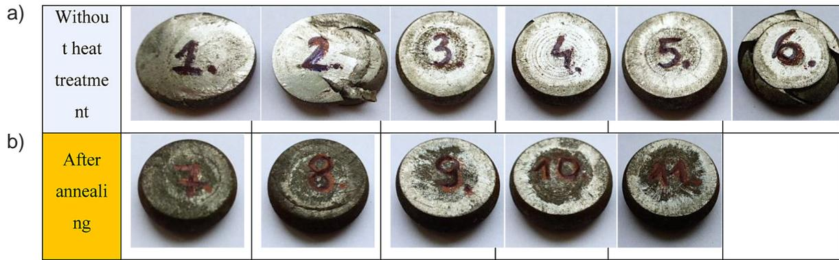
Fig. 3. Surfaces of steel specimens formed: a) without prior heat treatment, b) by annealing
