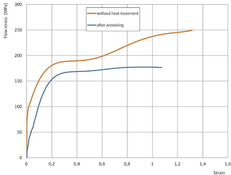
Fig. 4. Experimentally determined flow curves for cold formed 40HM steel: a) without heat treatment, b) after annealing
