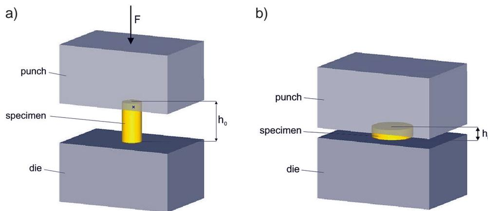
Fig. 2. Design of the compression test
