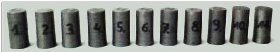
Fig. 1. Cylindrical specimens prepared for rolling
