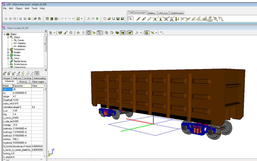
Fig. 1. Model of coal wagon type 12-757 of the Russian production with bogies 18-100 made in Universal Mechanism loco program
