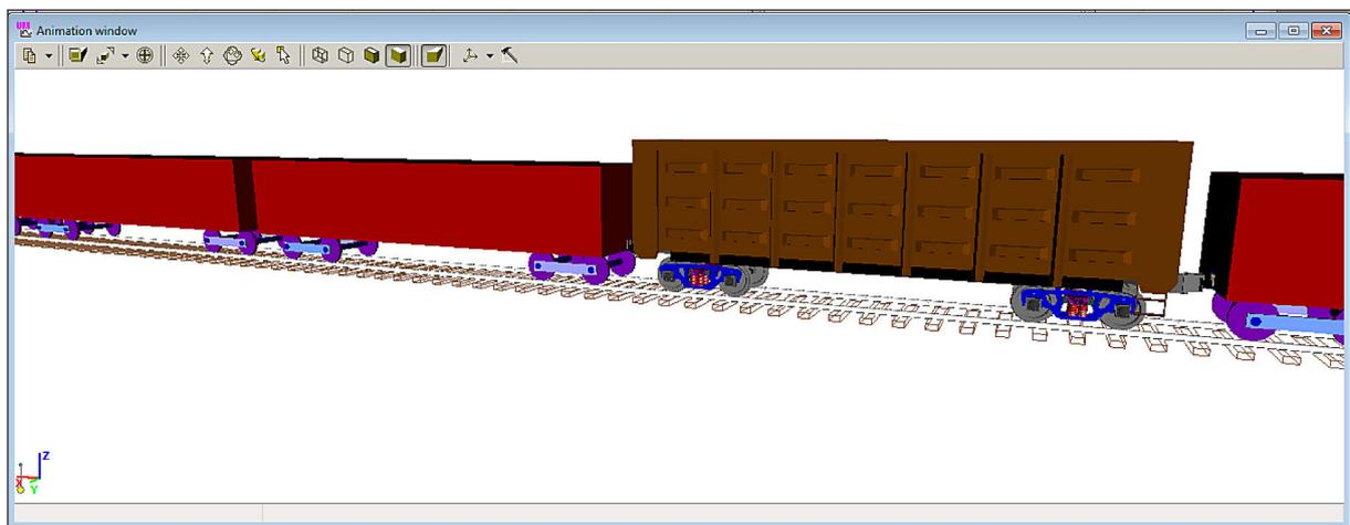
Fig. 9. View of portion of the model train with inserted wagon model 3D to determine the forces in the wheel/rail contact
