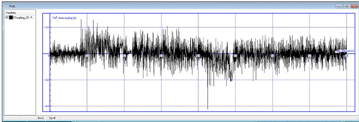
Fig. 10. The longitudinal force in compression coupling SA-3 in wagon No 33 (middle wagon)
