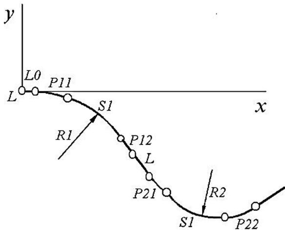
Fig. 6. Macro-geometry of railway line: L0, L – straight segment, P11, P12, P21, P22 – temporary curves, S1 – an arc of radius R1, H1 – superlevation of track, dy – widening of the track in the arc
