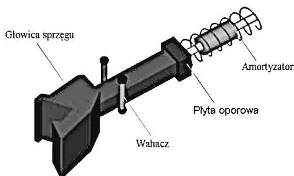
Fig. 3. Automatic coupler SA-3 along with frictional damper Sh-2-T [13]
