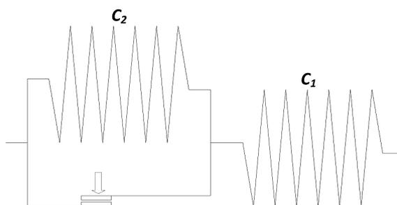
Fig. 4. Rheological model of SA-3 coupler C1, C2 - the stiffness of the springs
