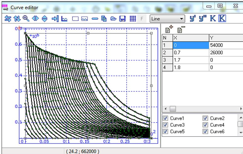
Fig. 5. Sample traction characteristics of electric locomotive
