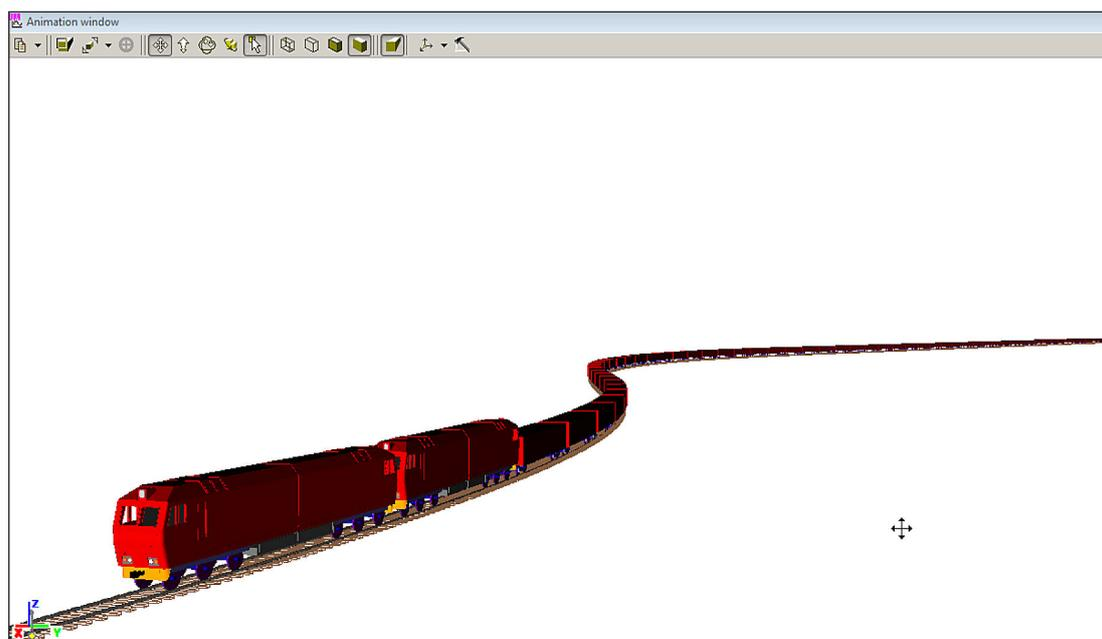
Fig. 2. Model of freight train made in UM program.
