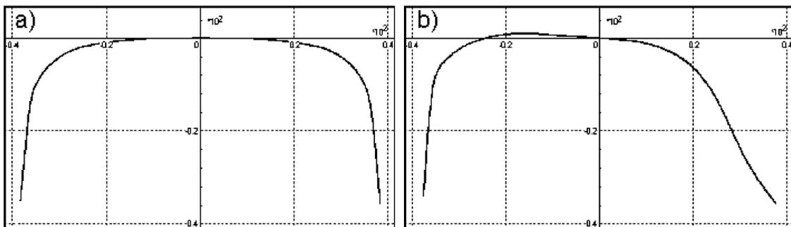
Fig. 8. Profile rail head type R65: a) new rail, b) splint worn unilaterally (external line of the arch rail road)
