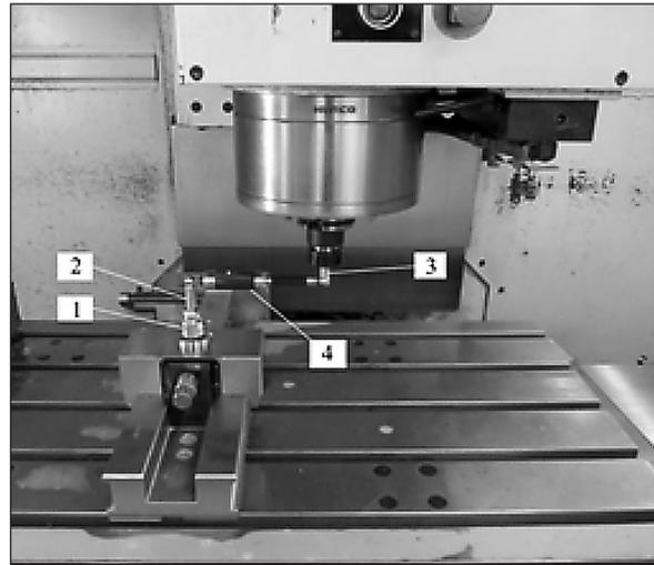
**Fig. 1.** Measuring device Ballbar QC20: 1 – Magnetic center holder, 2 – Magnetic centre cup attached to rack, 3 – Magnetic centre cup clamped in collet, 4 – Measuring device
