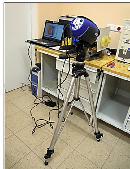
Fig. 8. Thermal imaging camera type FLIR SC5000
