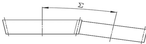
Fig. 4. Beveloid gear with spur gear
