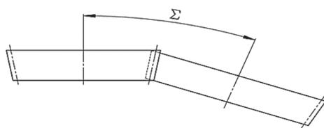
Fig. 5. Beveloid gears with angled axes
