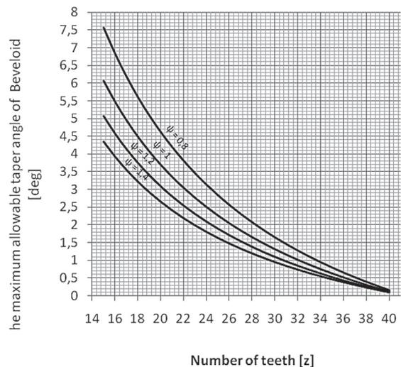
Fig. 6. Maximum allowable narrowing angle in Beveloid gears [deg]
