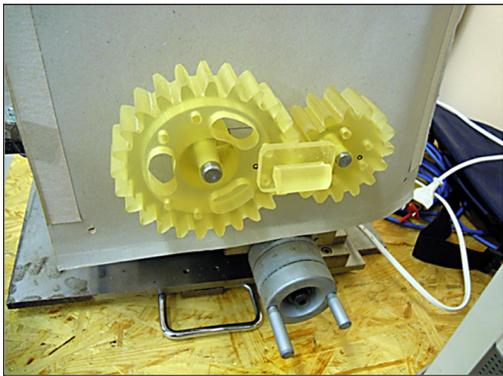
Fig. 9. The positioner of fine adjustment gears
