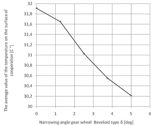
Fig. 12. The results of measurements, for the various gears, measured as the average surface temperature of gear mate
