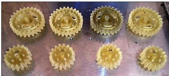
Fig. 10. Beveloid gears used in the experiment
