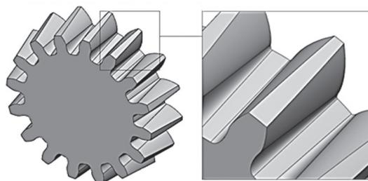
Fig. 2. The shape of the tooth space in Beveliod gear
