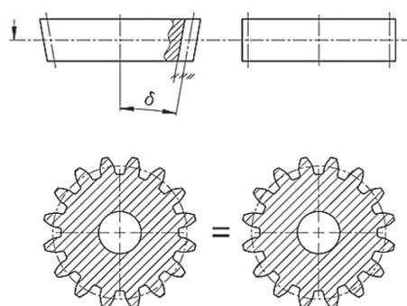
Fig. 1. Comparison of Beveliod gear geometry with a spur gear
