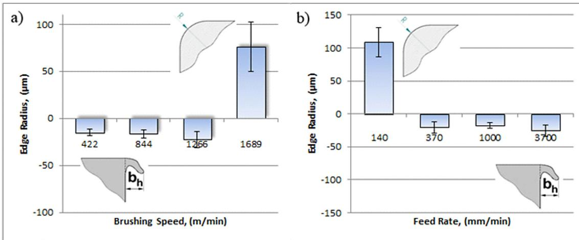
**Fig. 3.** Influence of brushing parameters upon edge radius for B1 brush: a) variable brushing speed, b) variable feed rate
