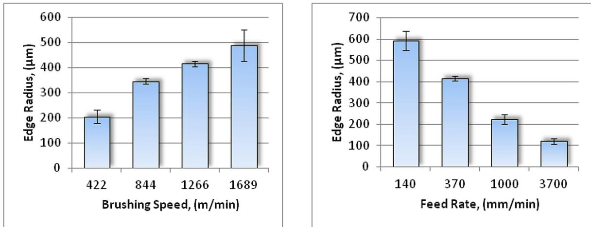
Fig. 4. Influence of brushing parameters upon edge radius for B2 brush: a) variable brushing speed, b) variable feed rate
