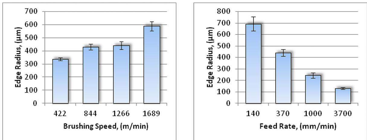
Fig. 5. Influence of brushing parameters upon edge radius for B3 brush: a) variable brushing speed, b) variable feed rate
