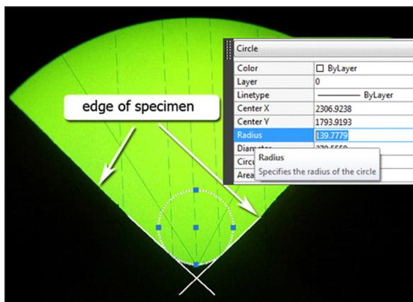
**Fig. 2.** Radius determining method
