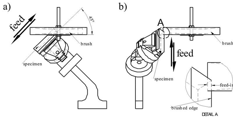
**Fig. 1.** Specimen orientation during brushing on a vertical machining center FV 580a: a) front view, b) side view
