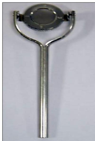
**Fig. 2.** Berthold's Magnetic Field Indicator
