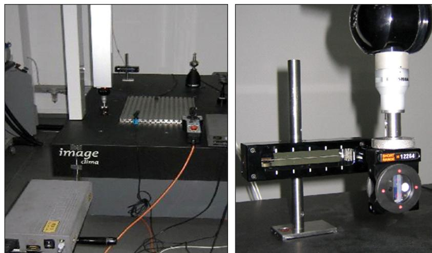
Fig. 2. Exemplary measurement of straightness errors using laser interferometer
