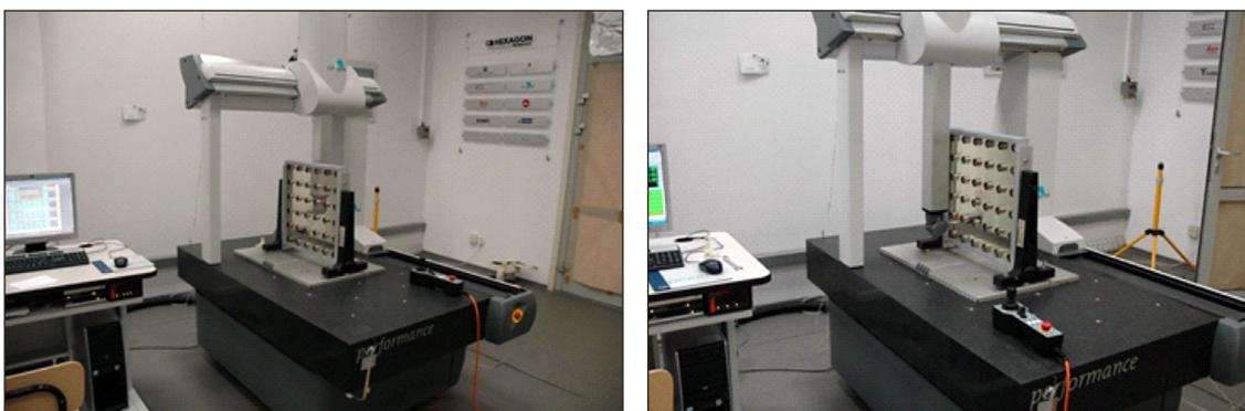
Fig. 3. Measurements of a hole plate in one of the positions recommended in Novel method [9]
