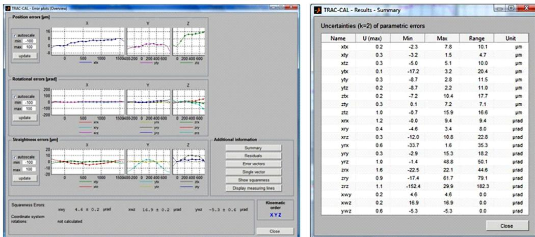
Fig. 7. Results of geometric errors identification using LaserTracer system
