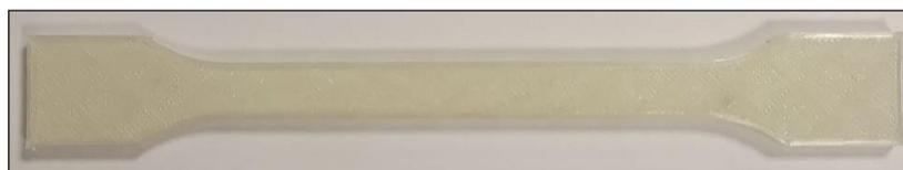
**Figure 5.** A sample for tensile strength test
