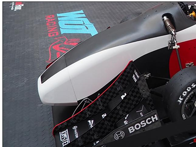
**Figure 1.** Front of the vehicle with nose cone and front wing
