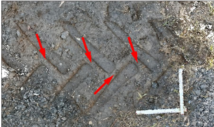
**Figure 9.** Trace in the sand, the red arrows indicate the places where the depth of the trace was measured
