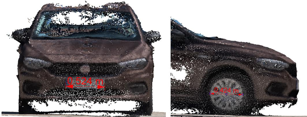
Figure 11. Verification dimensions for an intermediate scale object
