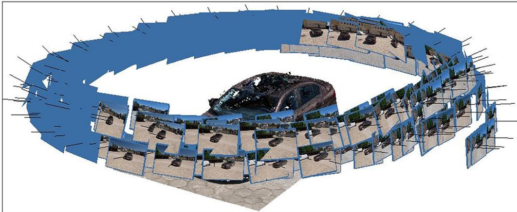
**Figure 2.** Example of taking photos of a car using a GoPro camera
