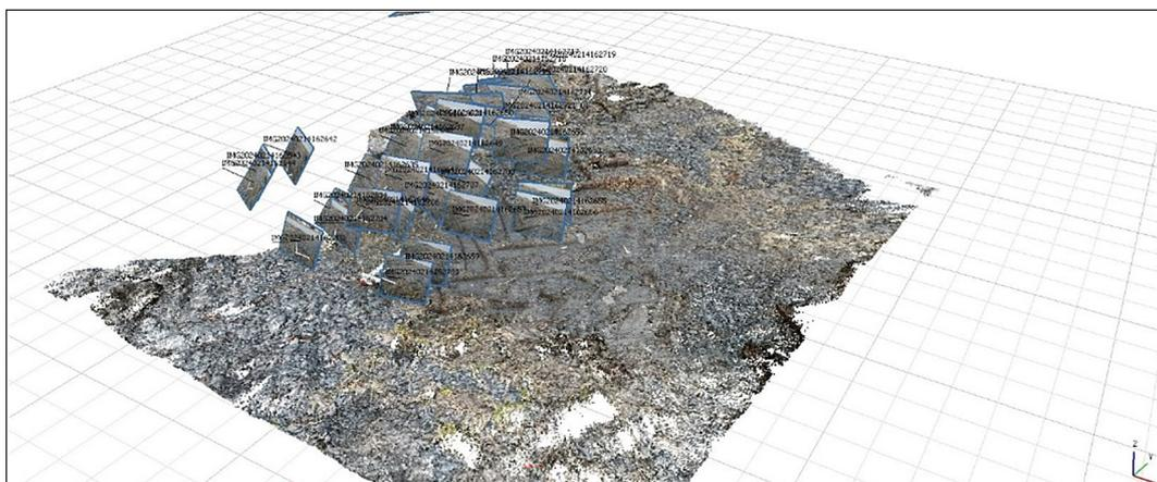
**Figure 1.** Example of taking photos of a tire tread impressed on the ground using a smartphone
