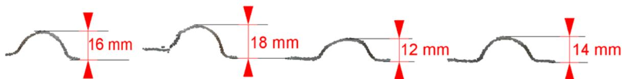
**Figure 10.** Measuring the depth of a trace on a point cloud
