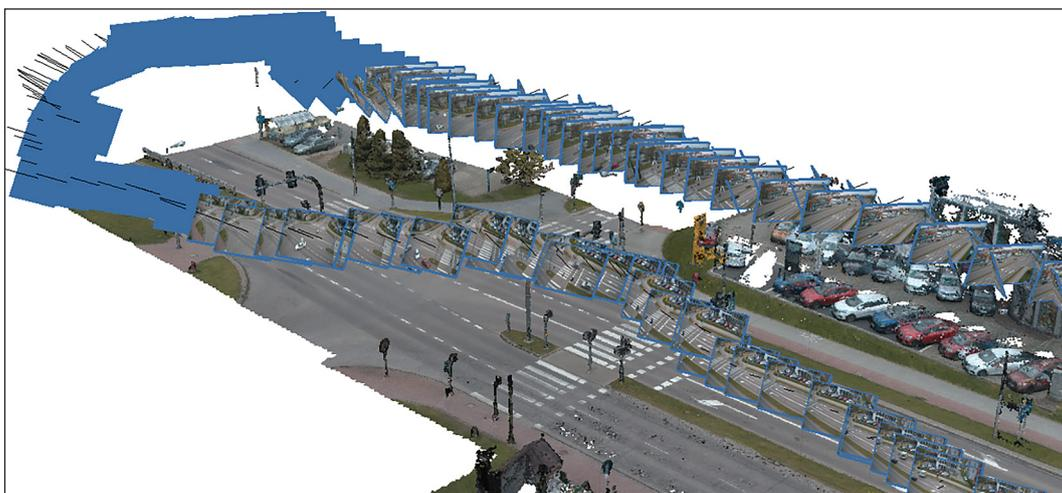
**Figure 3.** Example of taking photos of a road using a drone
