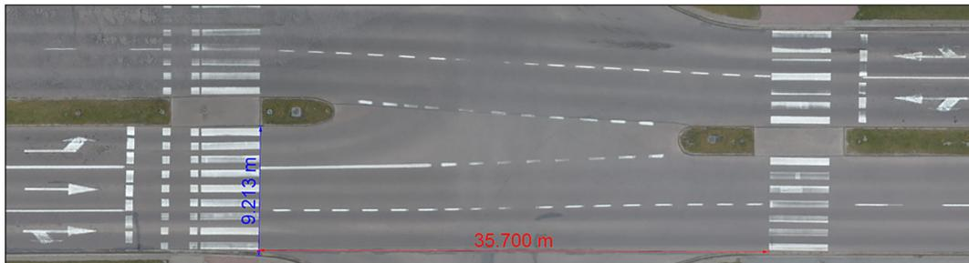
Figure 12. A point cloud representing a road; the red section is the reference dimension used for scaling, the blue section is the verification distance measured on the point cloud
