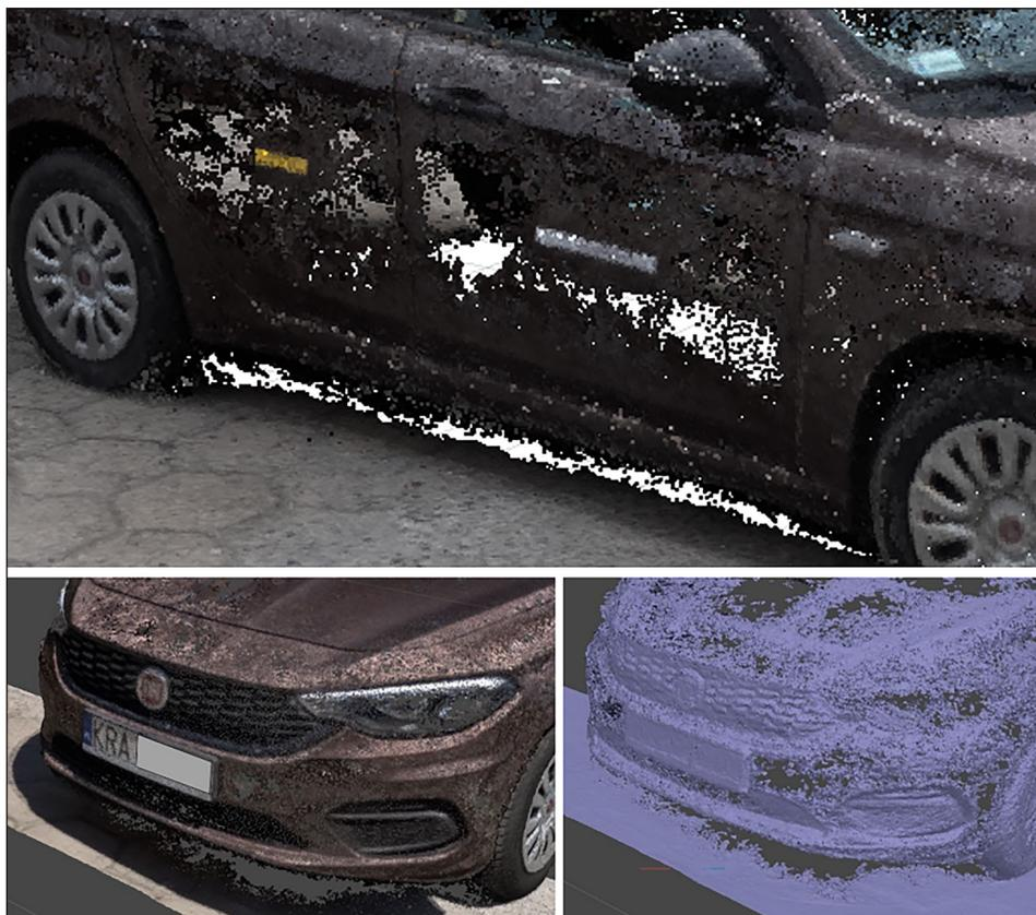
Figure 6. Filling point cloud discontinuities by using forensic scales (top) and fragment of the object's point cloud on an intermediate scale – multi-colored (left) and single-colored (right); photos were taken with a GoPro camera
