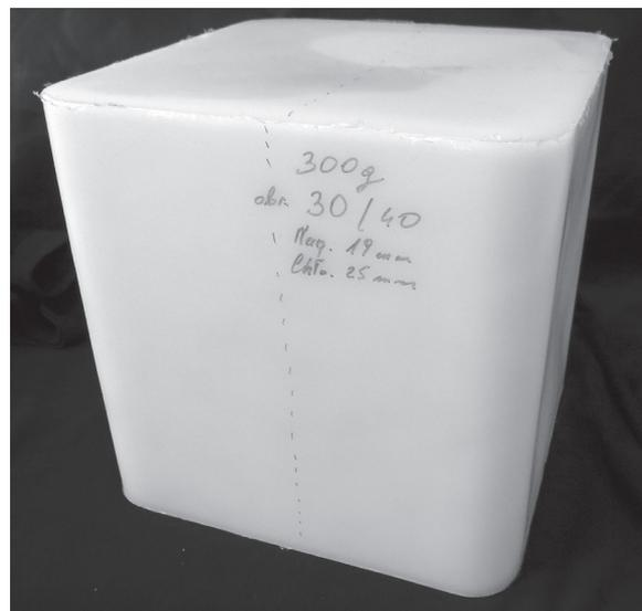
**Fig. 3.** Cast produced in rotational molding
