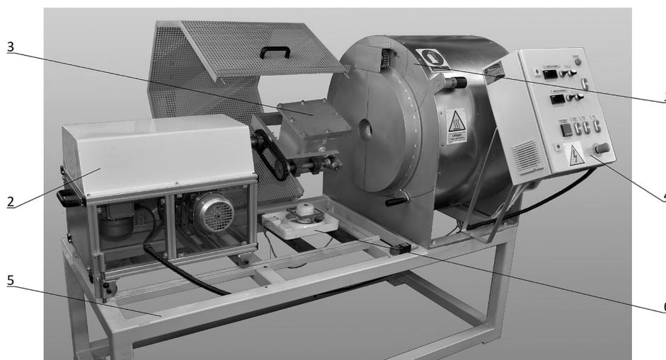
**Fig. 1.** Laboratory machine for rotational molding: 1 – heating system, 2 – rotational system, 3 – mold, 4 – control and regulation system, 5 – base, 6 – fan
