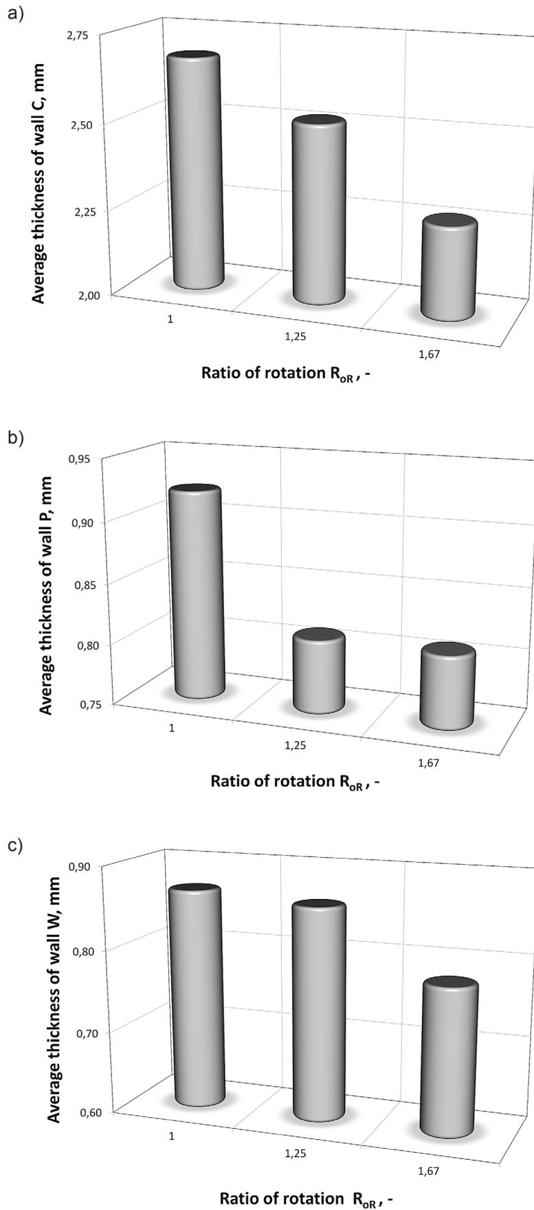
**Fig. 8.** Dependence of average wall thickness determined in geometric centre of cast on speed ratio  $R_{OR}$ : a) wall C, b) wall P, c) wall W
