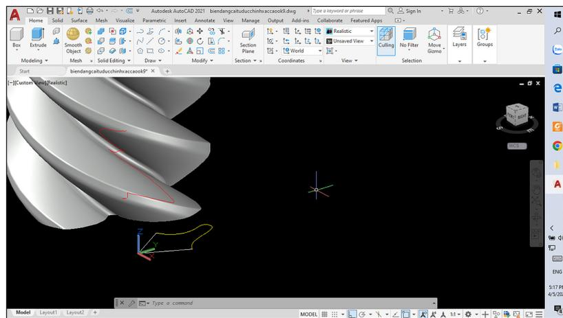
Figure 4. The gate rotor profile was created automatically
