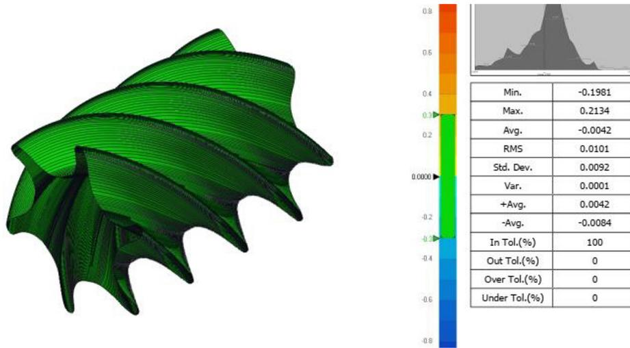
Figure 6. 3D surface comparison of two gate rotor surfaces generated by the two methods
