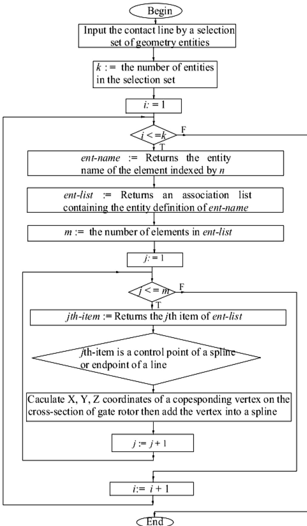
Figure 2. Algorithm of the Autolisp subroutine creating cross-section profile of the generated gear
