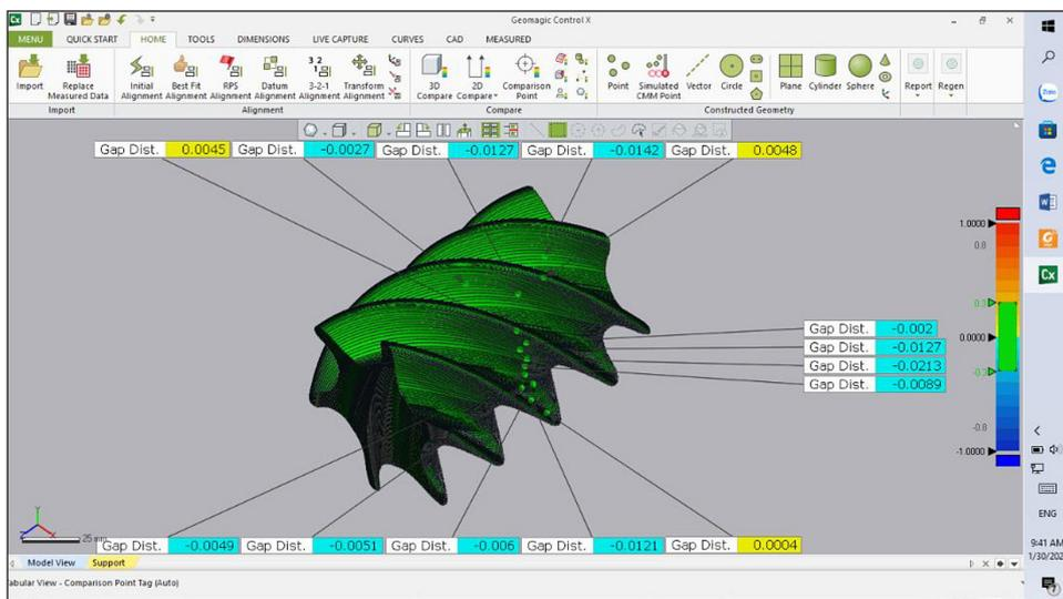
Figure 7. 3D point comparison of two gate rotor surfaces generated by the two methods
