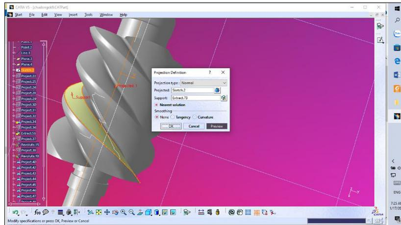
Figure 3. The contact line is created by the projection command in the CATIA
