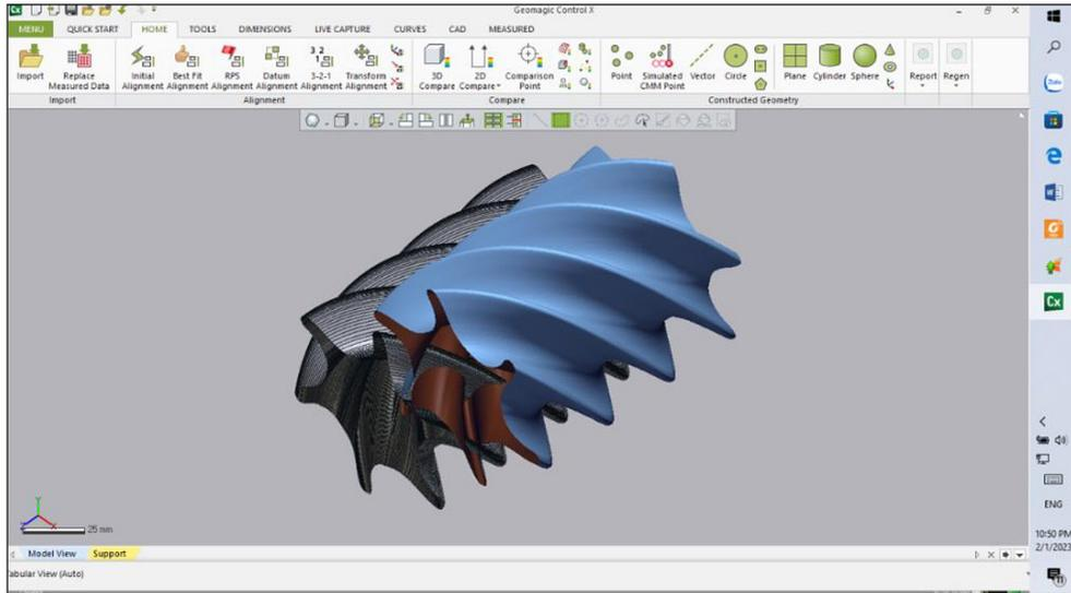
Figure 5. Two surfaces generated by the two methods are imported into the Geomagic.
