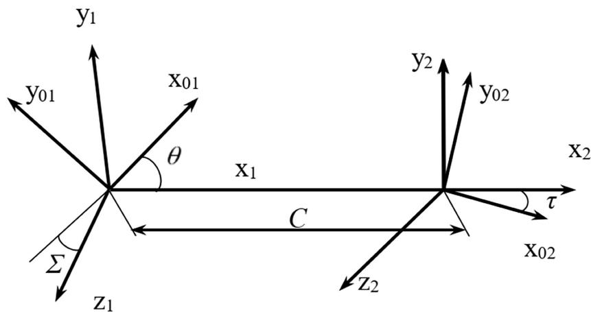
Figure 1. Coordinate systems of helical gears [2]
