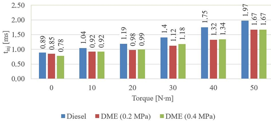
**Figure 3.** Differences in the fuel injection time values of diesel fuel and DME for different engine operating conditions ( $n = 950$  rpm) and with different supply pressures
