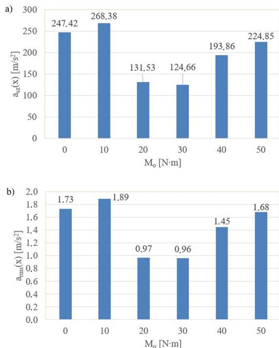
**Figure 10.** The influence of the combustion process of diesel fuel in the engine (fuel supply pressure: 0.2 MPa,  $n = 950$  rpm) on the averaged point estimates of the vibroacoustic process for the X direction (obtained for the time domain): (a) peak value of vibration accelerations ( $a_p$ ), (b) root mean square value of vibration accelerations ( $a_{rms}$ )
