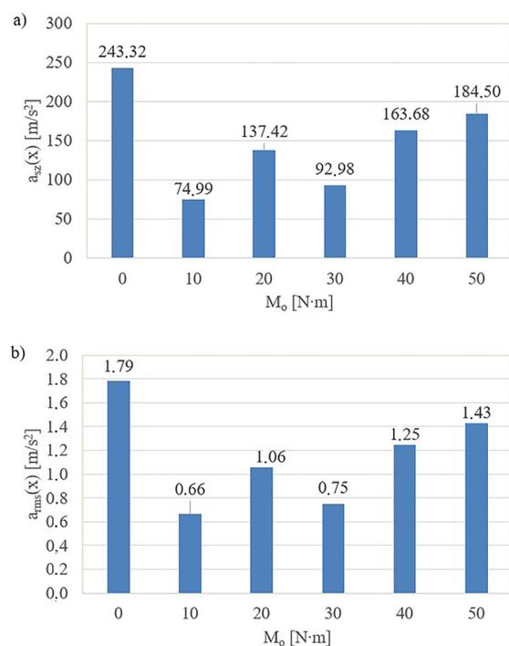
**Figure 11.** The influence of the combustion process of diesel fuel + DME in the engine (fuel supply pressure: 0.2 MPa,  $n = 950$  rpm) on the averaged point estimates of the vibroacoustic process for the X direction (obtained for the time domain): (a) peak value of vibration accelerations ( $a_p$ ), (b) root mean square value of vibration accelerations ( $a_{rms}$ )
