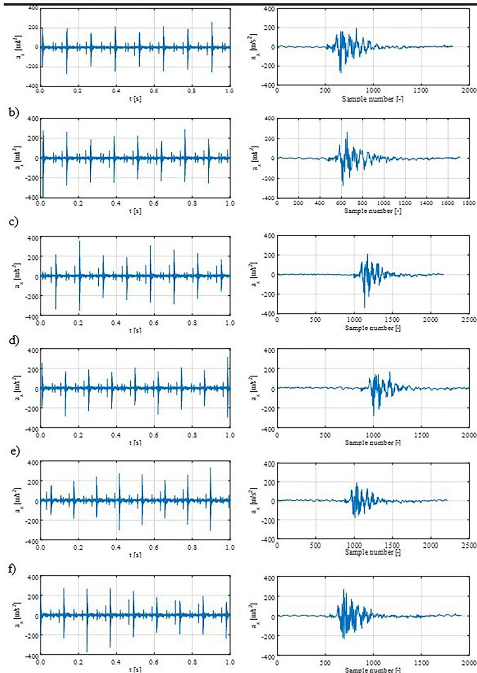
**Figure 8.** Time histories of vibration accelerations in the X direction ( $a_x$ ) and fragments for the combustion process of a diesel fuel in the engine obtained at  $n = 950$  rpm and  $M_o$ : (a) 0 N·m, (b) 10 N·m, (c) 20 N·m, (d) 30 N·m, (e) 40 N·m, (f) 50 N·m
