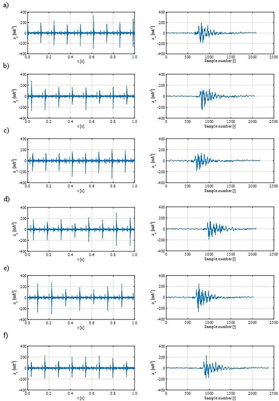
**Figure 9.** Time histories of vibration accelerations in the X direction ( $a_x$ ) and fragments for the combustion process of a diesel+DME fuel in the engine obtained at  $n = 950$  rpm and  $M_o$ :
