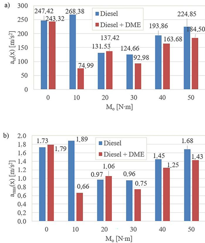
**Figure 12.** Comparison of the influence of the fuel type on the combustion run in the engine (fuel supply pressure: 0.2 MPa), mapped in the values of vibration acceleration in the X direction (obtained in the time domain) mapped for the averaged: (a) peak value ( $a_p$ ), (b) root mean square value ( $a_{rms}$ ), for different engine torques
