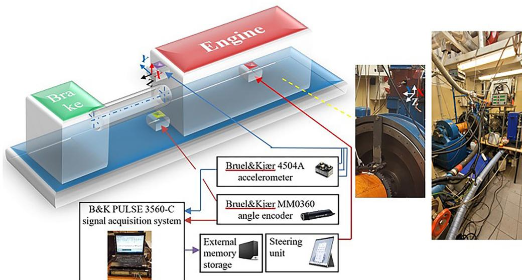
**Figure 2.** Type and arrangement of elements of the vibroacoustic measurement system for DME research
