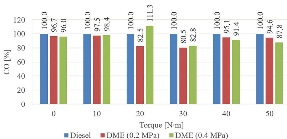
**Figure 6.** The influence of DME on the relative concentration of a carbon oxide (CO) in engine exhaust gases for different values of its torque and a supply pressure
