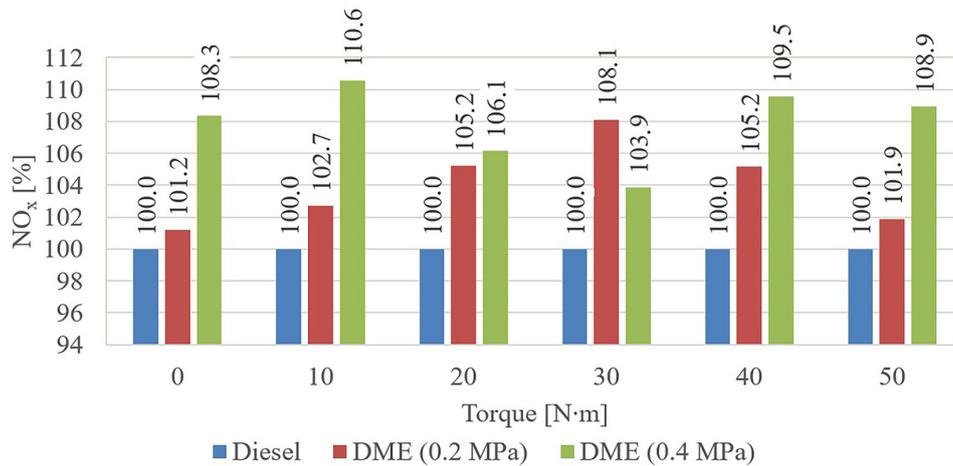
**Figure 7.** The influence of DME on the relative concentration of nitrogen oxides (NO<sub>x</sub>) in engine exhaust gases for different values of its torque and a supply pressure
