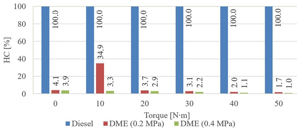
**Figure 4.** The influence of DME on the relative concentration of hydrocarbons (HC) in engine exhaust gases for different values of its torque and a supply pressure
