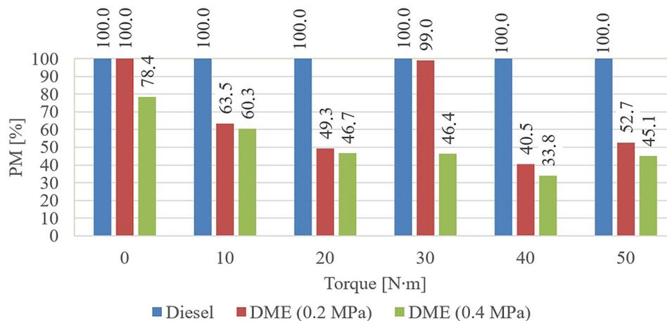
**Figure 5.** The influence of DME on the relative concentration of particulate matter (PM) in engine exhaust gases for different values of its torque and a supply pressure
