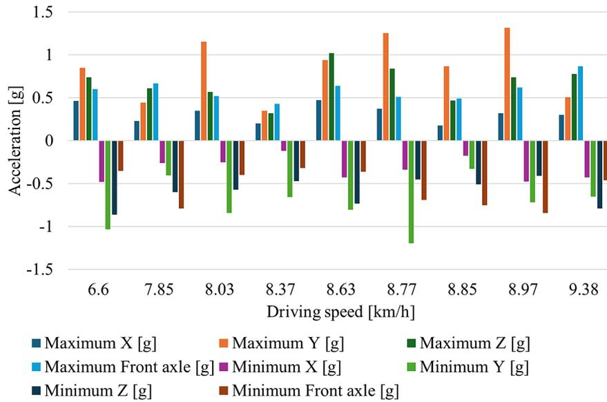
Figure 13. Maximum values of accelerations recorded in points no. 1–5 single obstacle road
