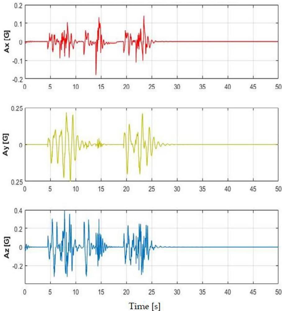
**Figure 11.** Time variation of accelerations measured by accelerometer number 5 while driving with a constant speed of 7.5 km/h
