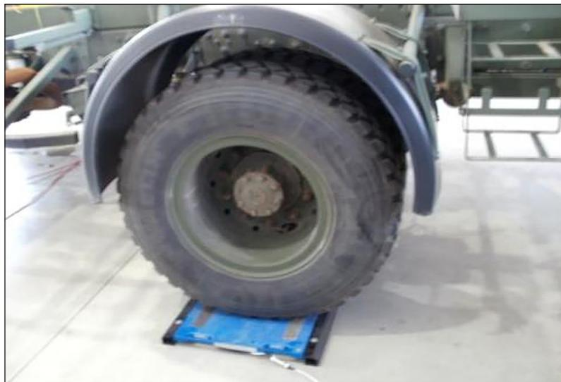
**Figure 7.** Weighing procedure for the truck rear axle
