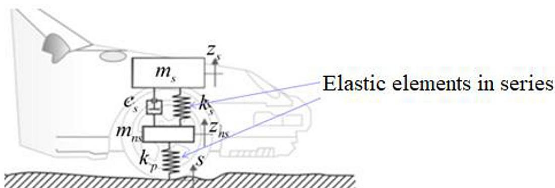
Figure 1. A diagram of the quarter-car model
