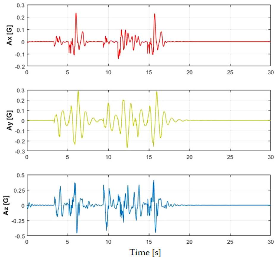
Figure 9. Time variation of accelerations measured by accelerometer number 5 while driving with a constant speed of 10 km/h
