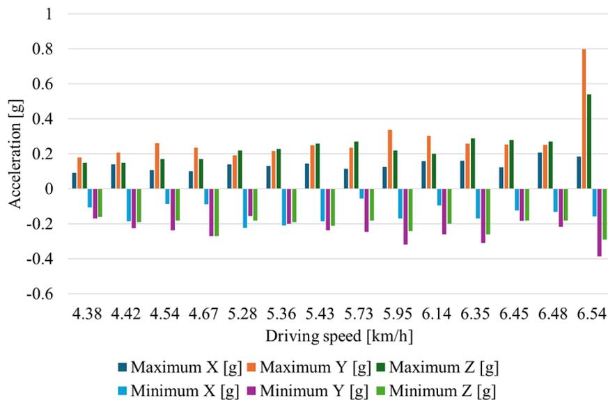
Figure 14. Maximum values of accelerations recorded in measuring point no. 5 for multiple obstacle road
