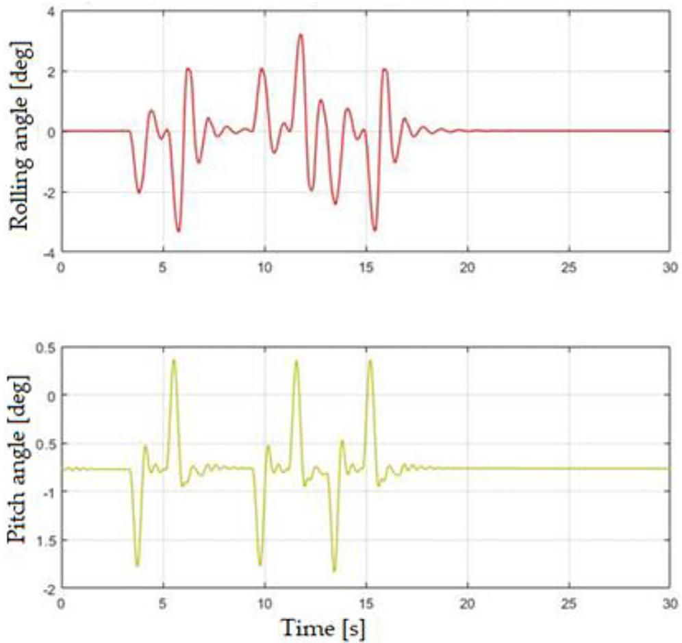
Figure 10. Time variation of rolling and pitch angle of the sprung mass
