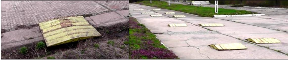
Figure 8. The layout of obstacles for single obstacle road (a) and multiple obstacle road (b)
