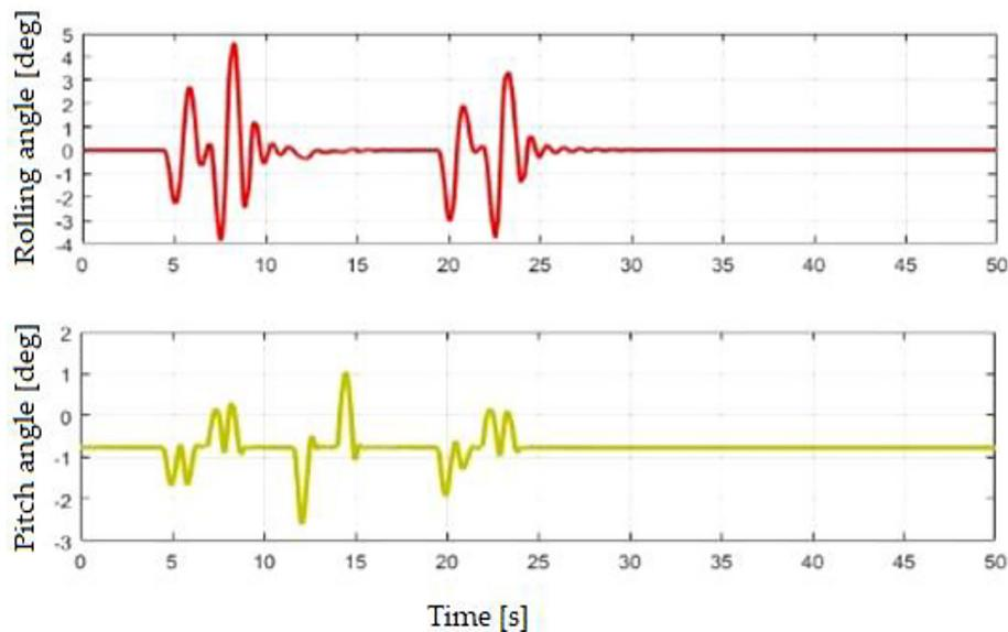
Figure 12. Time variation of rolling and pitch angle of the sprung mass
