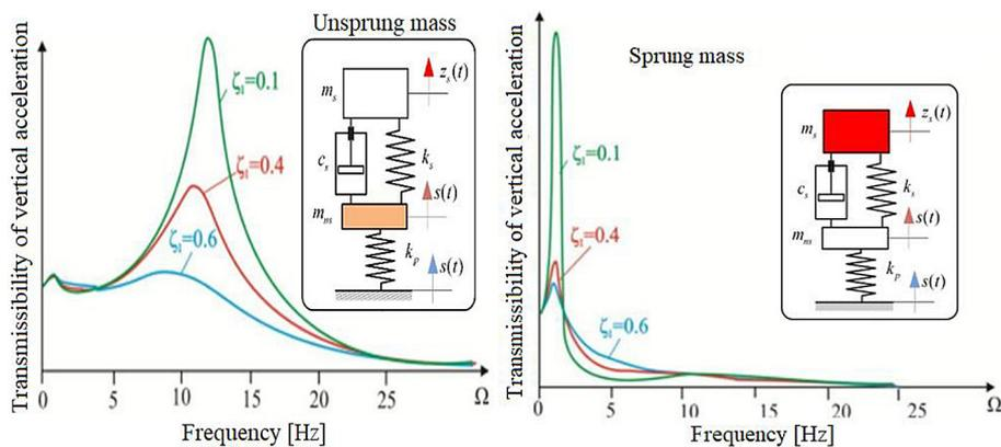
Figure 2. Transmissibility characteristics for elastic elements in series (a) and for sprung mass (b)
