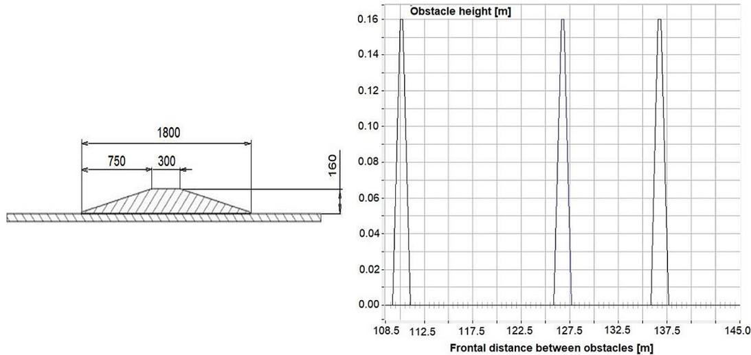
**Figure 4.** Parameters of the obstacles for single obstacle size (a) and 2d shape of modelled track (b)
