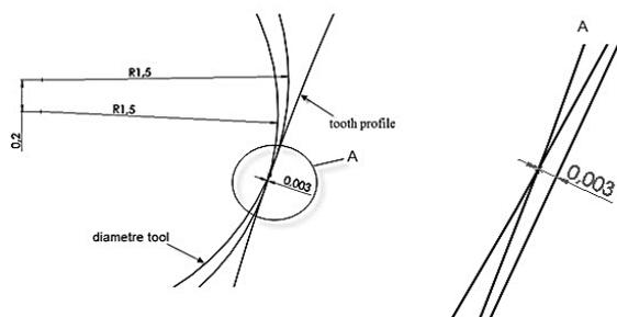
**Fig. 5.** The milling cutter profile during the manufacturing process and its deviation (in millimeters)
