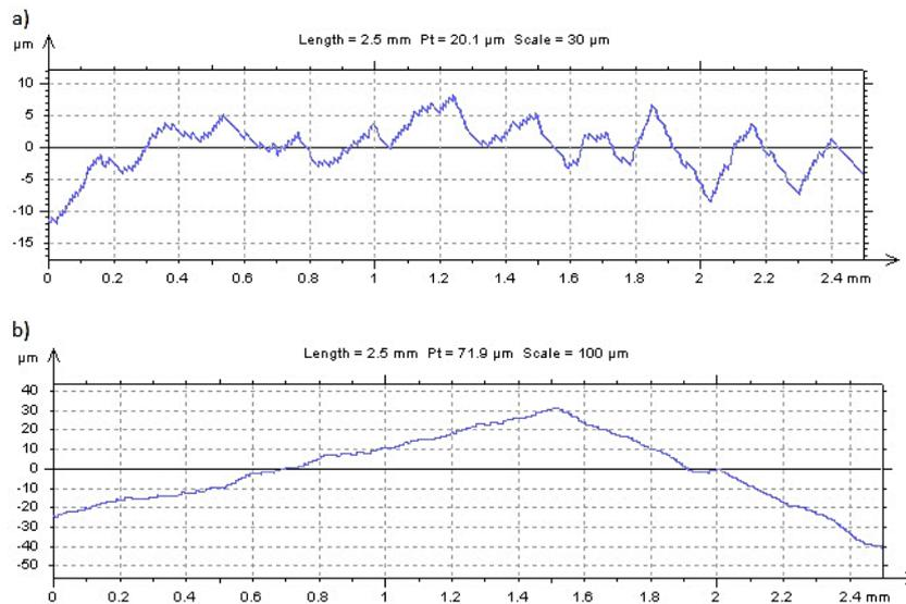
**Fig. 4.** The roughness profiles measured along the tooth profile: a) 15-teeth gear, b) 17-teeth gear
