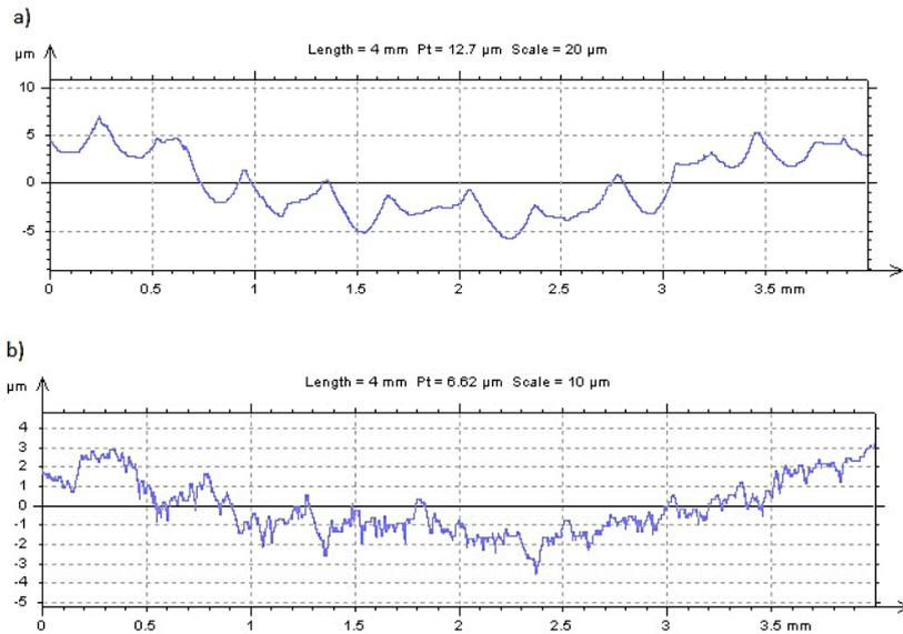
**Fig. 3.** The roughness profiles measured along the tooth line: a) 15-teeth gear, b) 17-teeth gear
