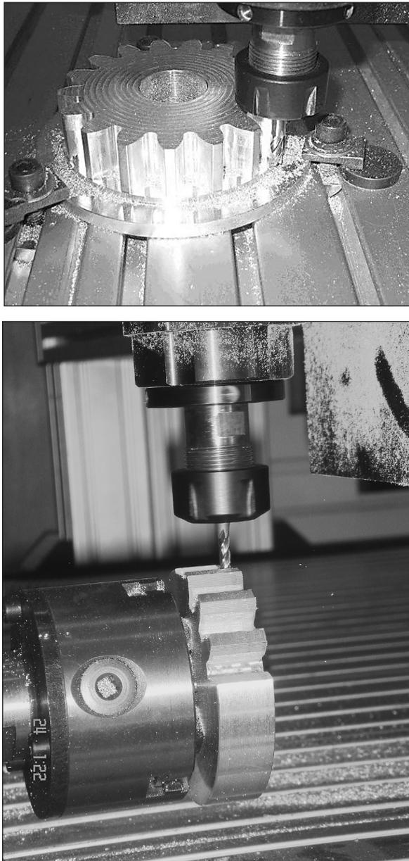
**Fig. 1.** The methods of gears manufacturing on the universal machine tool
