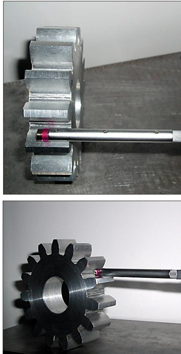
**Fig. 2.** The measurement of gear roughness on Surtronic 3+
