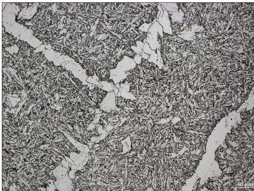
**Figure 3.** Microstructure of the as-cast steel composed of  $\delta$  ferrite in the shape of bright with grains,  $\alpha$  ferrite formed from the austenite as small grains and small amount of martensite
