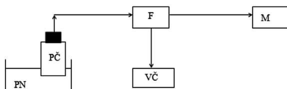
**Fig. 3.** Schematic connection of the Flowtronic device into the fuel system: PN – fuel tank, PČ – fuel pump, F – Flowtronic 205, VČ – evaluating component, M – engine.
