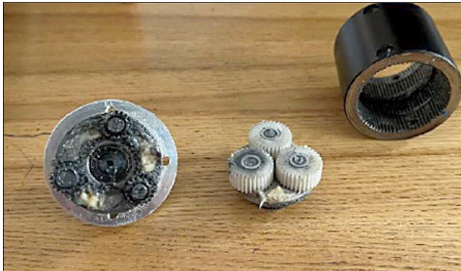
**Figure 2.** Two stages of the planetary gear of Diam57 NEMA23 motor
