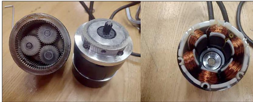
Figure 7. NEMA 23 BLDC motor after dismantling the housing and exposing the windings. Visible residual insulation level of the windings (on the right)
