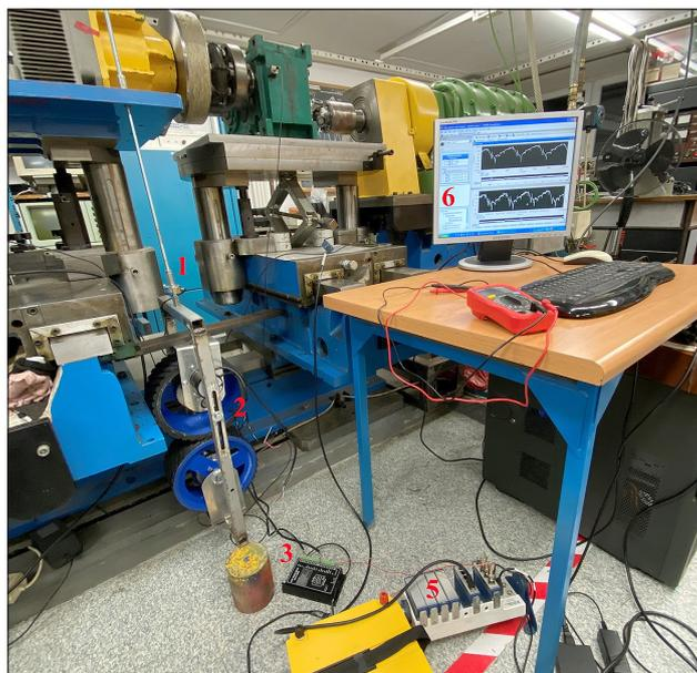
**Figure 4.** Test stand in laboratory conditions: 1 – KMM20 strain gauge load cell, 2 – rolling resistance test bench (Fig. 5), 3 – BLD-300B motor controller, 4 – 24V lithium-ion battery, 5 – NI eDAQ-9178 chassis for measurement systems with a multi-channel module equipped with NI 9234 and NI 9237 analogue-to-digital converters, 6 – PC with LabView Signal Express software
