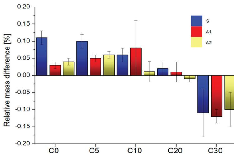
Figure 17. Differentiation in mass after salt crystallization process
