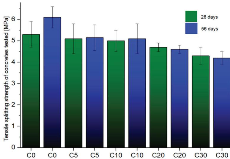
Figure 9. Tensile splitting strength of the concretes tested
