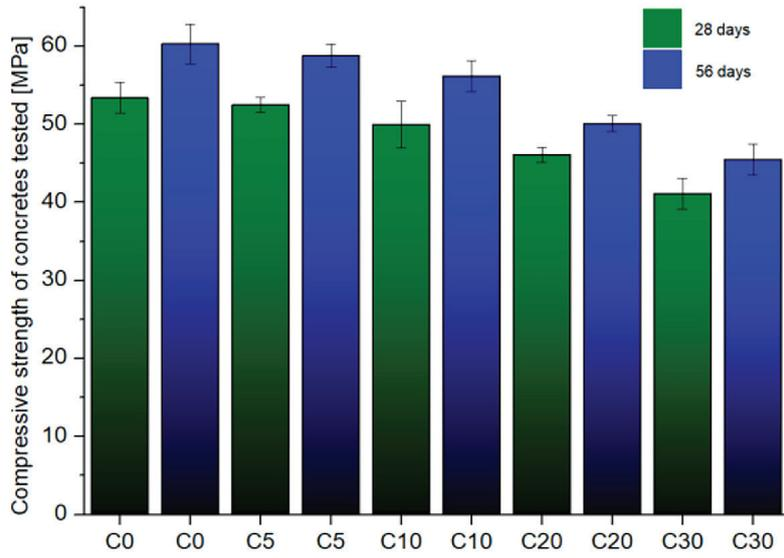
Figure 8. Compressive strength of the concretes tested
