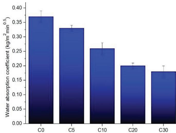
Figure 7. Water absorption coefficient of the concretes tested
