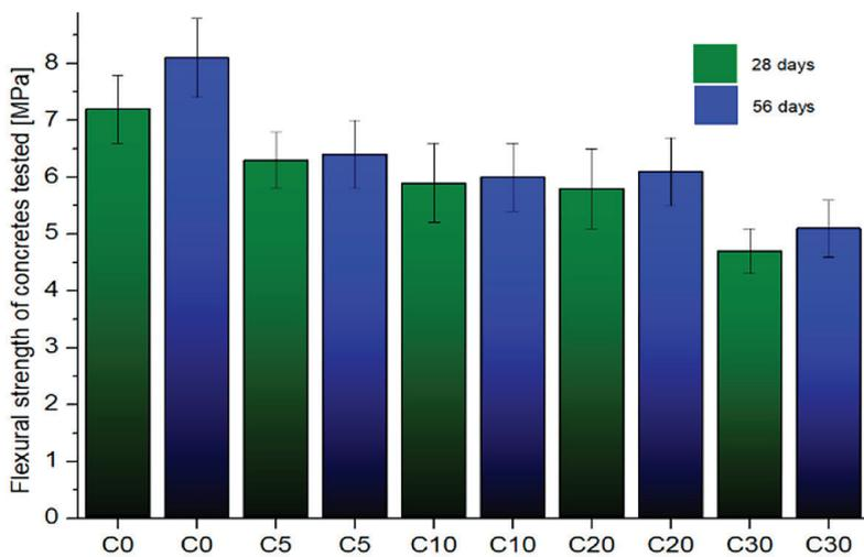
Figure 10. Flexural strength of the concretes tested
