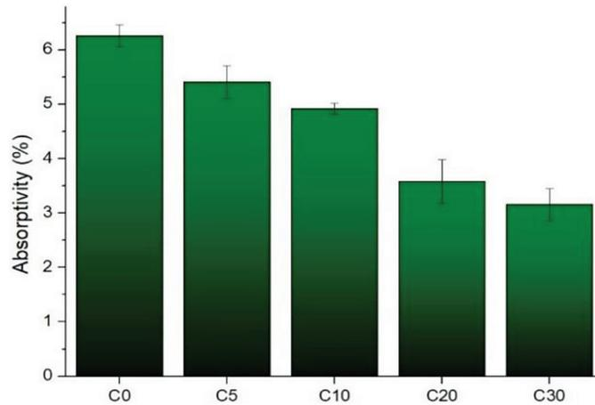
Figure 6. Absorptivity tested concretes
