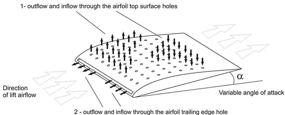
Fig. 1. Diagram illustrating the main objectives of the project
