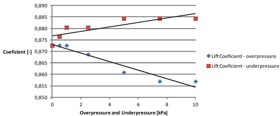
Fig. 7. Lift coefficient for different values of overpressure and vacuum
