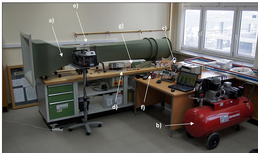
Fig. 2. Wind tunnel test bench for airfoils with active airflow
