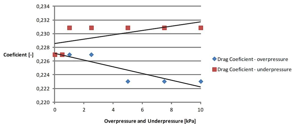
Fig. 8. Drag coefficient for different values of overpressure and vacuum
