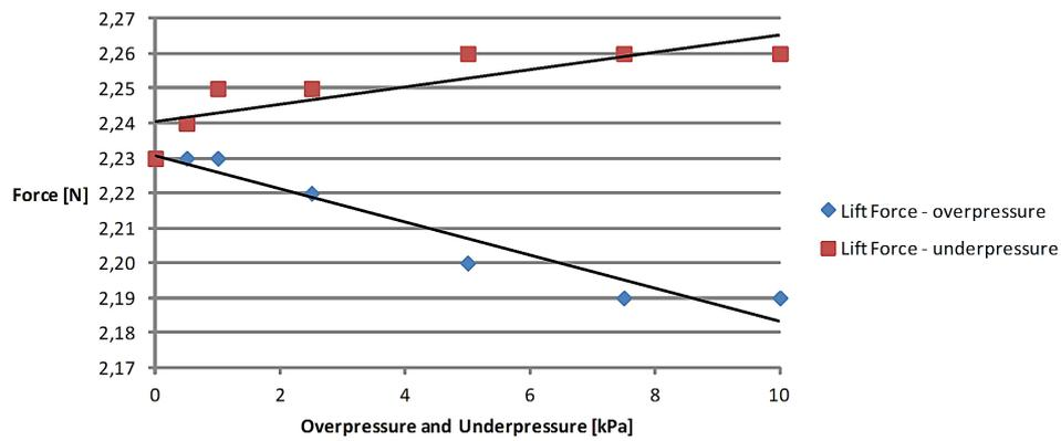
Fig. 5. Lift force for different values of overpressure and vacuum
