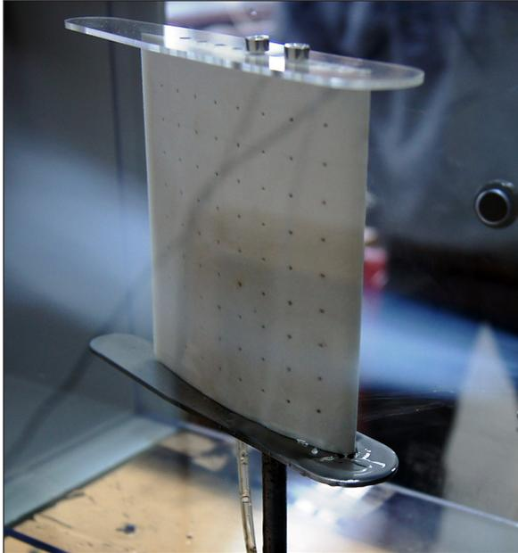
Fig. 4. Ready airfoil mounted in the wind tunnel
