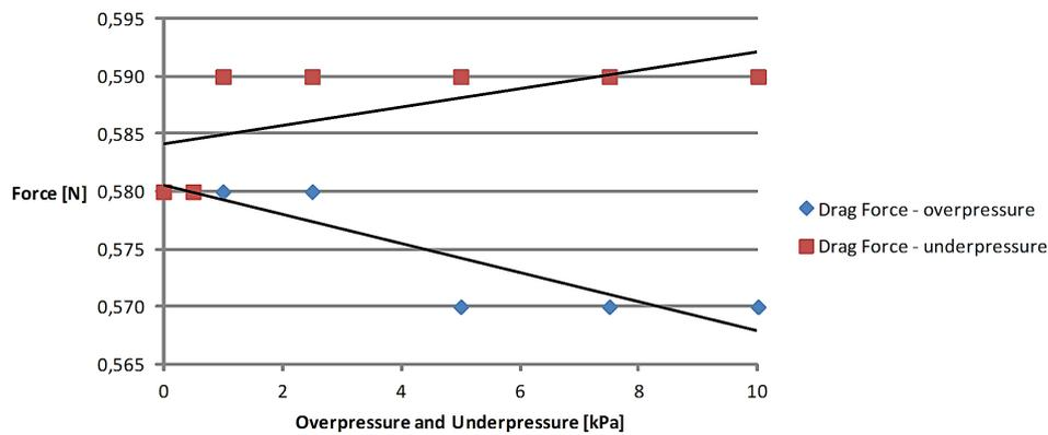
Fig. 6. Drag force for different values of overpressure and vacuum
