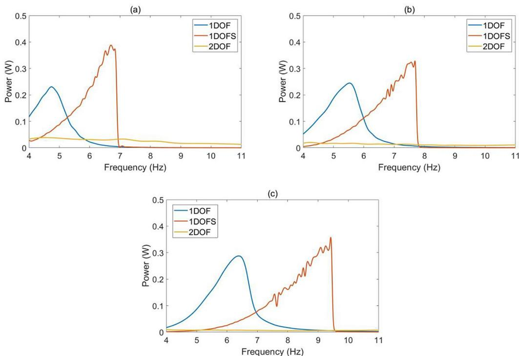
**Figure 5.** Recovered instantaneous power versus excitation frequency obtained from three harvester configurations: (a)  $b = 160$  mm, (b)  $b = 150$  mm and (c)  $b = 140$  mm. The amplitude of the shaker’s excitation was 0.8 g
