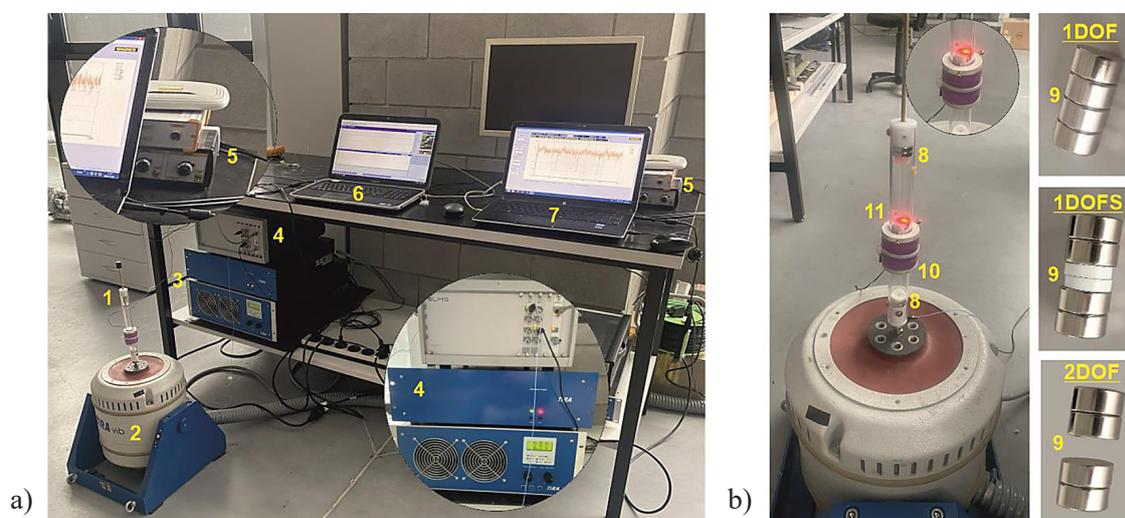
**Figure 2.** The experimental setup: (a) and electromagnetic harvester mounted in the electro-magnetic shaker with various oscillating magnets (b)
