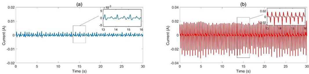
**Figure 8.** Current output from the 1DOF harvester for moving speeds: (a) 5 km/h and (b) 13 km/h
