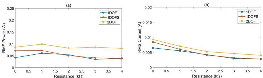
**Figure 12.** RMS: (a) power and (b) current from various energy harvesters concepts at different load resistances, for a moving speed of 9 km/h and horizontal gradient of the treadmill
