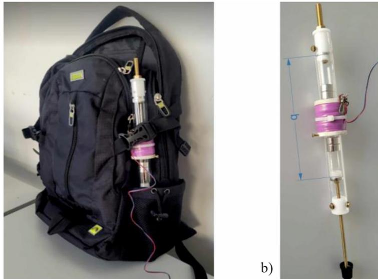
**Figure 3.** (a) Energy harvesting backpack and (b) 2 DOF electromagnetic harvester
