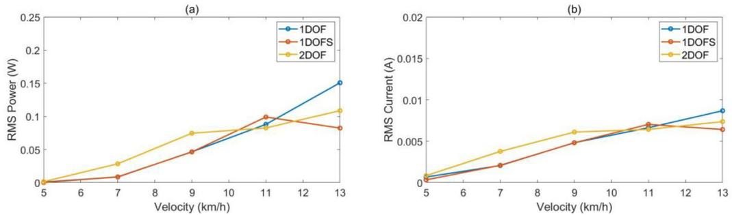
**Figure 11.** RMS: (a) power and (b) current from various energy harvester concepts at different moving speeds, for a load resistance of 1 kΩ and horizontal gradient of the treadmill
