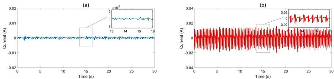
**Figure 9.** Current output from the 1DOFS harvester for moving speeds: (a) 5 km/h and (b) 13 km/h
