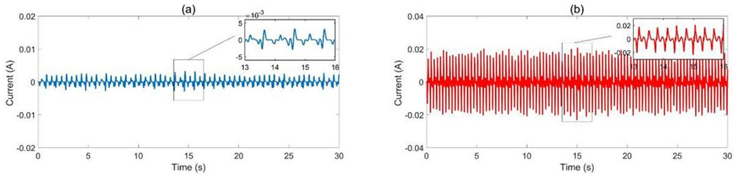
**Figure 10.** Current output from the 2DOF harvester for moving speeds: a) 5 km/h and b) 13 km/h
