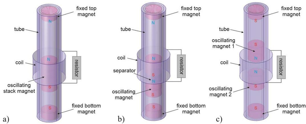
**Figure 1.** Three designs of electromagnetic harvesters: (a) 1DOF, (b) 1DOF with separator (1DOFS), and (c) 2DOF
