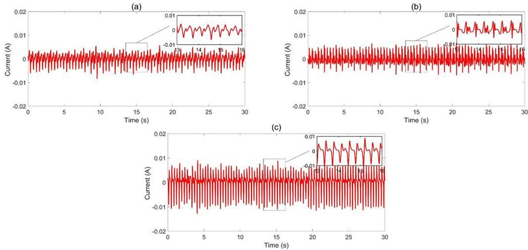
**Figure 7.** Instantaneous power obtained from three harvesters: (a) 1DOF, (b) 1DOFS and (c) 2DOF. The tests were conducted with a load resistance of 1 kΩ and in a horizontal treadmill setting
