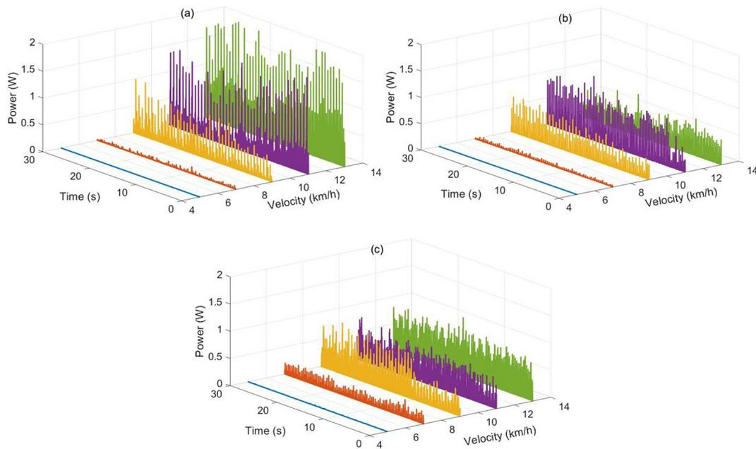
**Figure 6.** Instantaneous power obtained from three harvesters: (a) 1DOF, (b) 1DOFS and (c) 2DOF. The tests were conducted with a load resistance of 1 k $\Omega$  and in a horizontal treadmill setting
