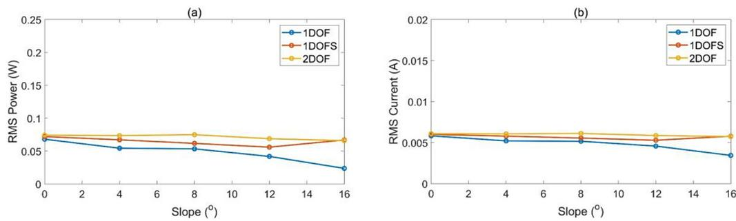
**Figure 13.** RMS: (a) power and (b) current from various energy harvesters at different treadmill slopes, for a moving speed of 9 km/h and a load resistance of 1 k $\Omega$
