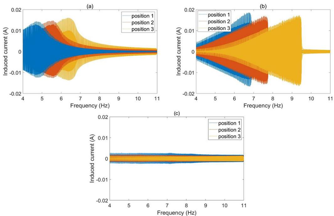
**Figure 4.** Frequency sweep responses obtained from three harvesters: 1DOF (a), 1DOFS (b), and 2DOF (c) for three different magnetic suspensions. The amplitude of the shaker's excitation was 0.8g. The blue line represents the separation between the fixed end magnets  $b = 160$  mm, the orange line for  $b = 150$  mm, and the yellow for  $b = 140$  mm
