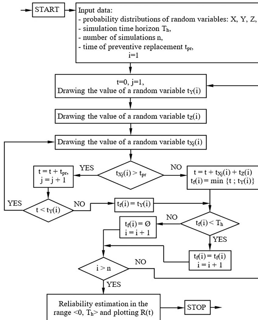
**Figure 5.** Block diagram of a simulation with a preventively renewed rubber damper element
