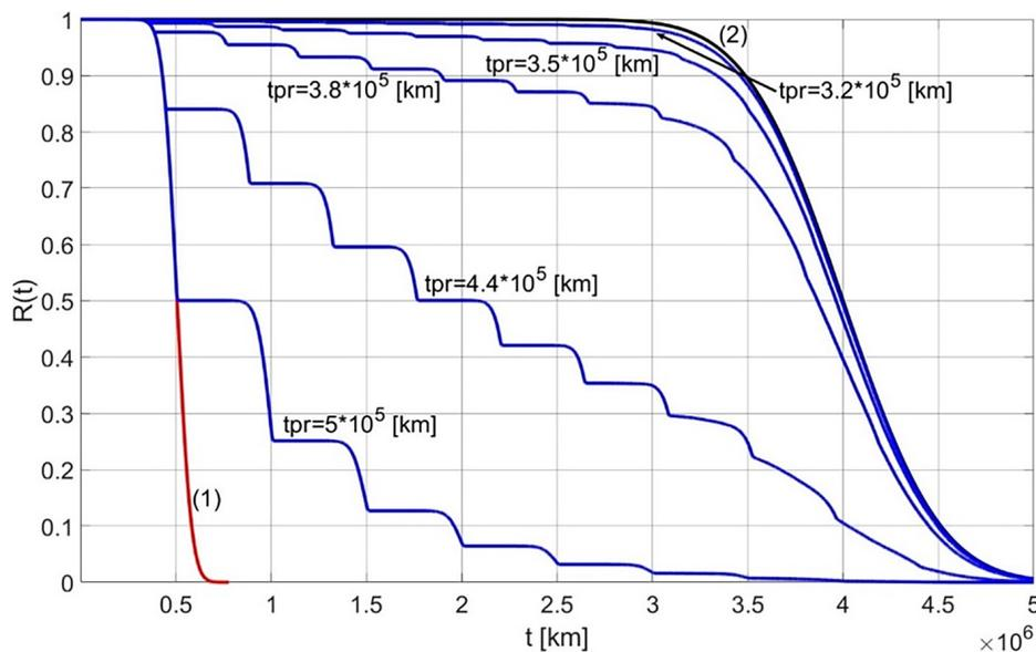
Figure 6. Reliability of the pivot-damper system with preventive renewal of the damper rubber element
