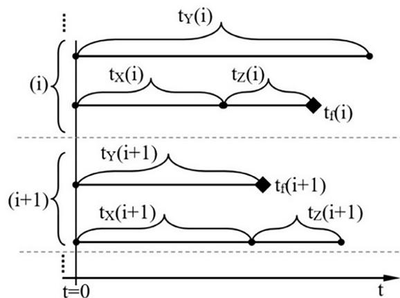
**Figure 2.** Determination of operating time to system failure ( $t_f$ ) in simulations
