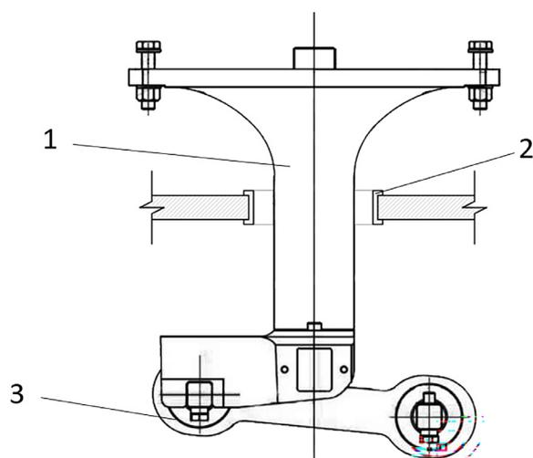
**Figure 1.** Schematic diagram of the construction of the analysed rail vehicle bogie pivot system, 1 – rail vehicle bogie pivot, 2 – through-port of the rail vehicle bogie frame cross member, 3 – tractive force vibration damper (metal-rubber bushing)
