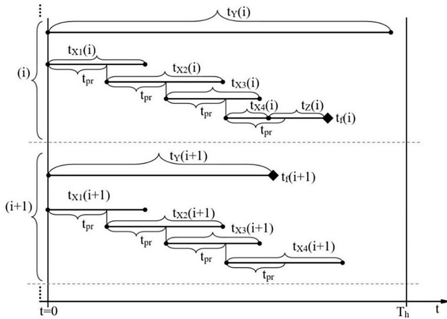
**Figure 4.** Determination of the operating time to system failure ( $t_f$ ) in simulations when the rubber element of the damper is renewed preventively at intervals  $t_{pr}$
