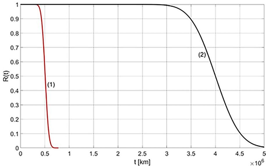
**Figure 3.** Reliability of the pivot-rubber element of the damper (1) and the course of the reliability of the system if the rubber element of the damper did not fail (2)
