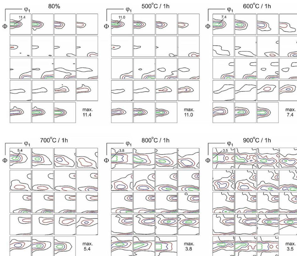
**Figure 7.** Orientation distribution function (ODFs) for austenite after 80% deformation and annealing at temperature 500–900 °C for 1 hour
