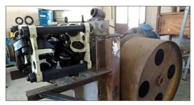
Figure 2. The wire rolling equipment utilized in the present study
