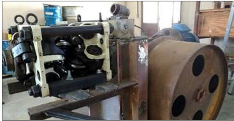
**Figure 2.** The wire rolling equipment utilized in the present study
