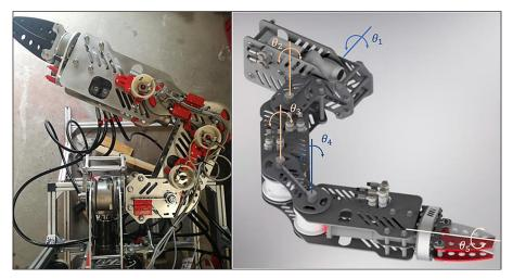
Figure 8. The real manipulator and its CAD model with the description of rotation angles  $\theta_1$ ,  $\theta_2$ ,  $\theta_3$ ,  $\theta_4$ ,  $\theta_5$
