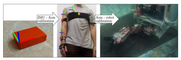
Figure 1. Idea of a human-machine interface that allows the robot to be controlled by the operator's hand using IMU sensors
