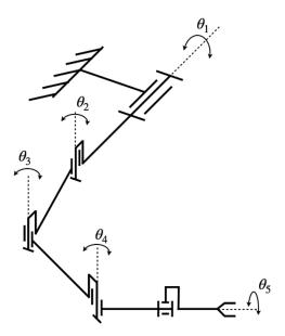
Figure 9. The manipulator kinematic scheme
