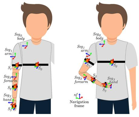
Figure 2. Proposal of placing of IMU sensors on the operator's body in the system modeling the movement/orientation of hand parts
