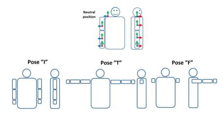
Figure 4. Schematic illustration of the calibration items required in the "IMU-arm" calibration process
