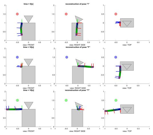
**Figure 7.** Visualization of the reconstructed positions from the measurement sequence (Figure 5) after the calibration process (Figure 6) with calibration matrices X, Y, Z, V (4) for three selected times: t = 5s for position "I", t = 10s for position "T" and t = 16s for position "F"
