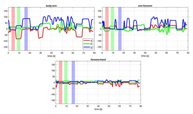
Figure 6. Courses of relative orientation angles of individual pairs of members of the kinematic chain of the operator's hand reconstructed after the "IMU-arm" calibration process
