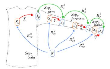
Figure 3. Schematic model of the association of the IMU measuring sensors and members of the kinematic chain of the operator's arm
