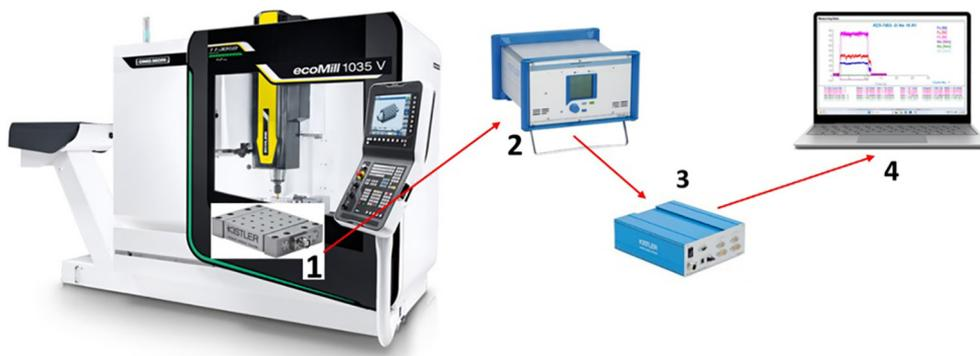
Fig. 4. Cutting force measurement bench: 1- Kistler 9199AA force sensor, 2- Kistler 5070A signal amplifier, 3- Kistler 5697A data acquisition system, 4 – PC with DynoWare 2825D software
