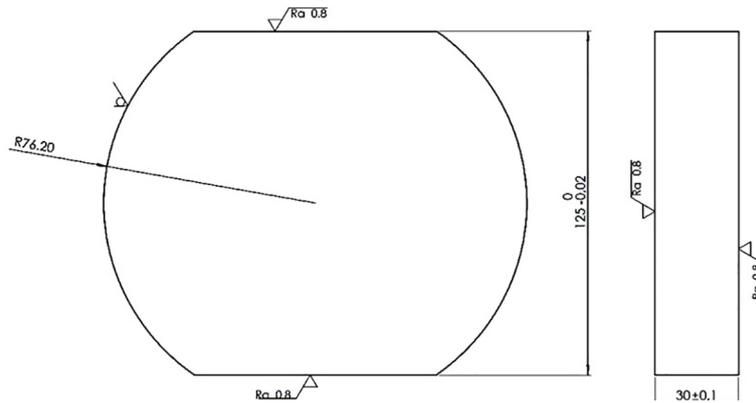
Fig. 2. A sample for testing made of Inconel 718
