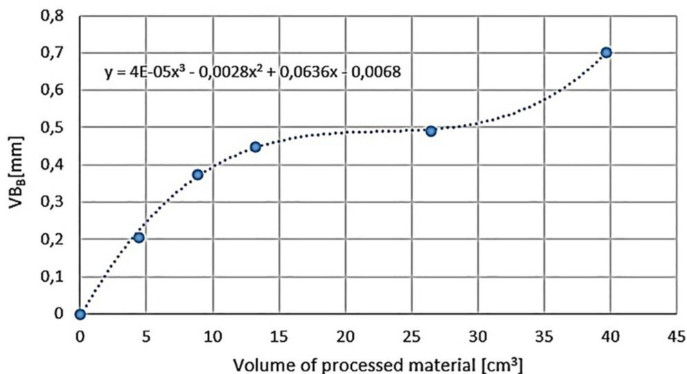
**Fig. 7.** Diagram of the dependence of cutting edge wear ( $V_{BB}$ ) on the volume of machined material for high feed milling with CS300 insert for machining parameters:  $v_c = 800$  m/min,  $f_z = 0.5$  mm/edge,  $a_e = 70.54$  mm,  $a_p = 0.5$  mm
