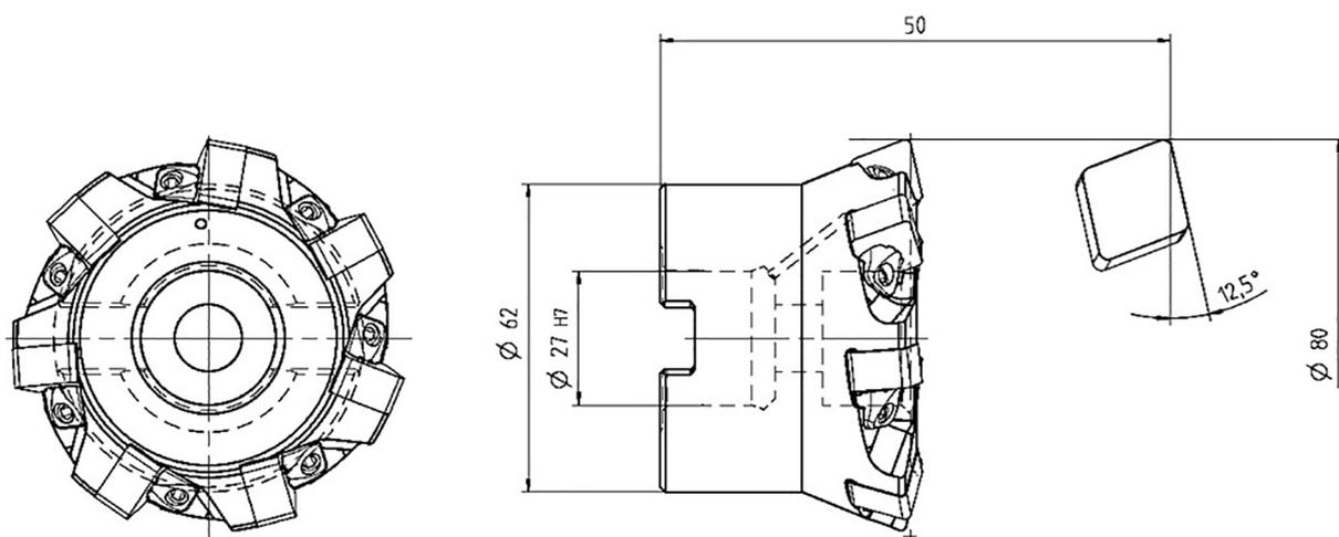
Fig. 1. Designed milling head
