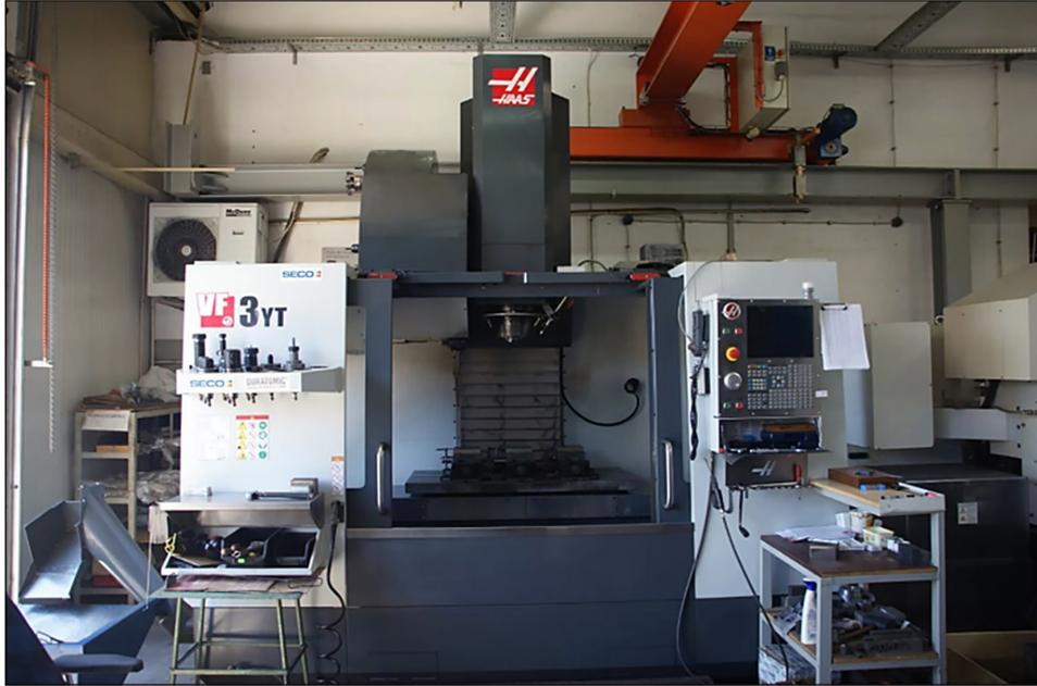
Fig. 6. HAAS VF3/YT milling center used for machining tests
