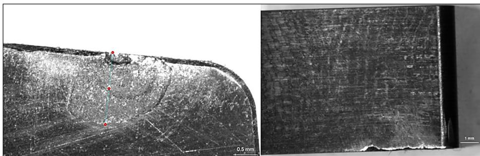
Fig. 5. Microscope image of the flank face of the CS300 insert for high feed milling (optical magnification 0.5x). Microscope image of the rake face of the CS300 insert for high feed milling (optical magnification 1.6x)
