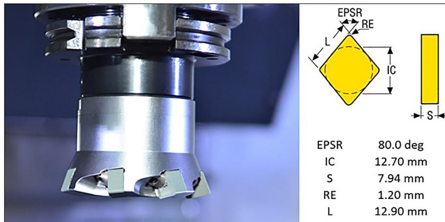
Fig. 3. Designed milling head with CNGN120712 inserts, mounted in the spindle of the milling center
