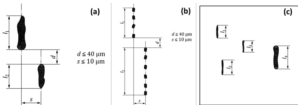
Fig. 5. Various inclusion types (a) A and C types inclusions, (b) B type inclusion (c) D type inclusions [45]
