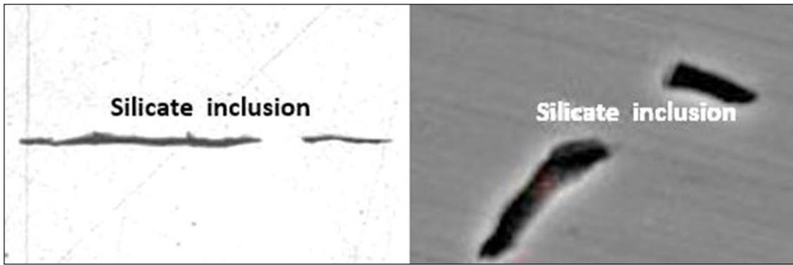
**Fig. 4.** Typical morphology of silicate inclusions
