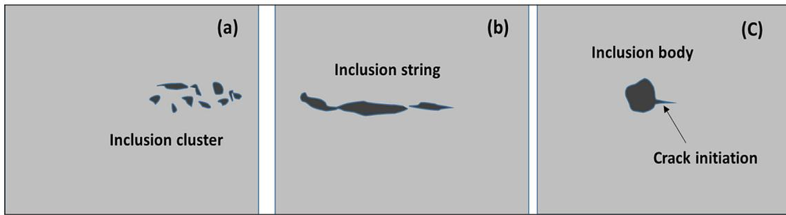
**Fig. 2.** Schematic of oxides inclusions (a)  $\text{Al}_2\text{O}_3$ , (b)  $\text{SiO}_2\text{,Al}_2\text{O}_3$ , and (c)  $\text{Al}_2\text{O}_3\text{,CaO}$
