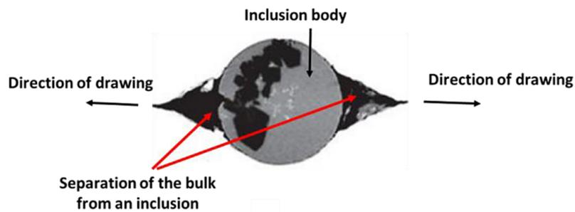
Fig. 6. Cold drawing steel wire created voids at the ends of a hard, massive, non-deformable NMI – adapted from [47]
