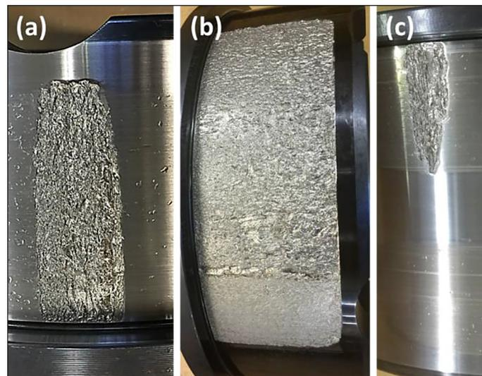
**Fig. 1.** Fractography of three failed bearings by fatigue (a) uncoated single row cylindrical roller bearing, (b) failed bearing coated with black oxide, (c) double row uncoated failed bearing
