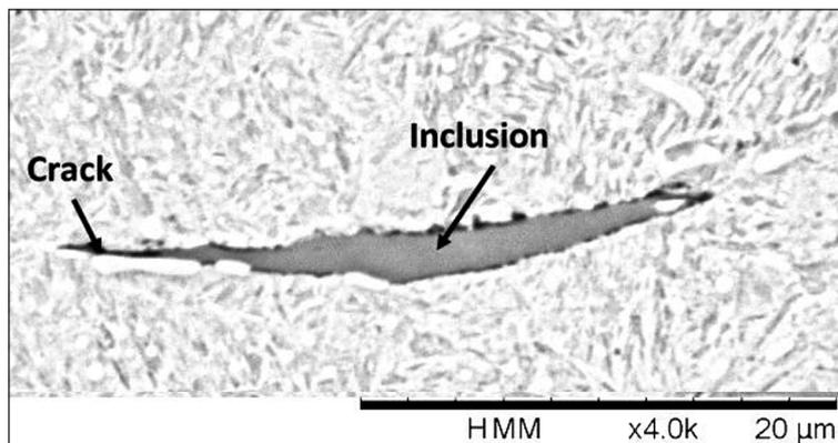
**Fig. 3.** A large  $\text{MnS}$  inclusion present in a hardened steel microstructure
